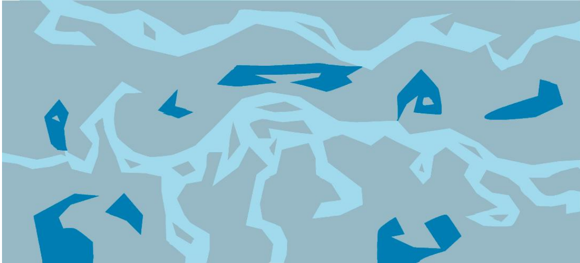
Figure 12 - Effective porosity—only the connected pores (light blue) can transmit water; the unconnected pores (dark blue) are not a part of the effective porosity.
