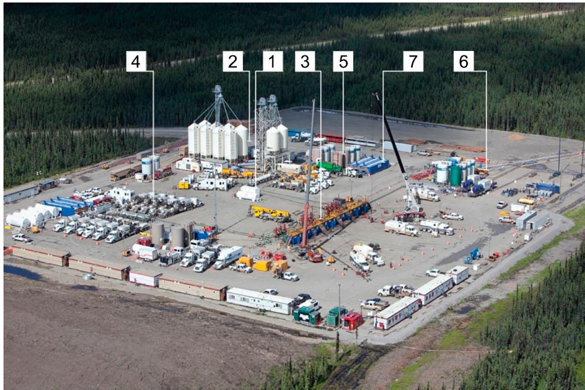
Figure 14 - Surface infrastructure of a well-pad site during hydraulic fracturing stimulation ("fracking"). Source: Council of Canadian Academies, 2014 (photograph courtesy of Nexen Energy, ULC). The numbered labels are as follows.
