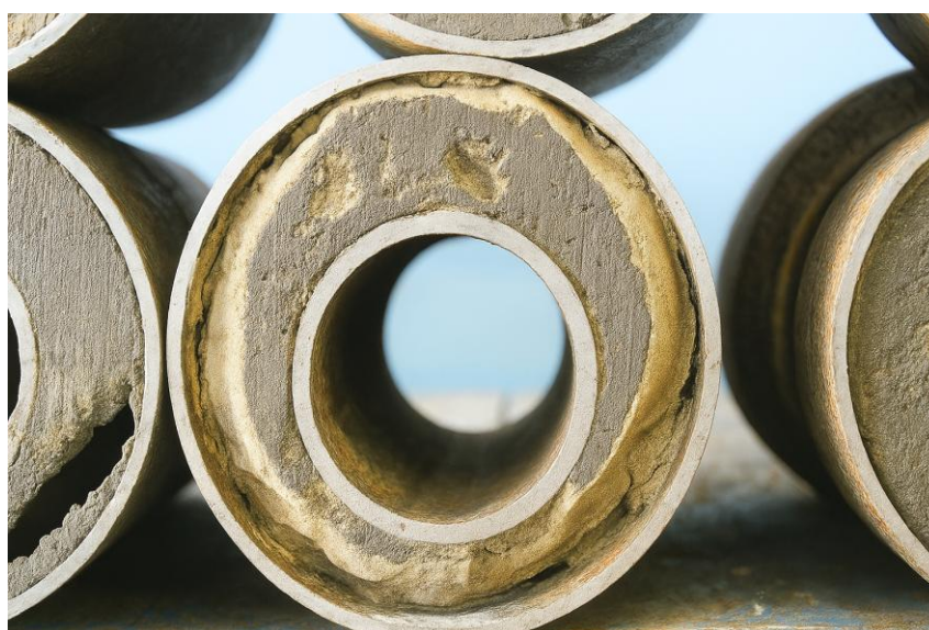
Figure 4 - Cement and drilling fluid channels resulting from incomplete drilling mud displacement because the casings are eccentrically aligned rather than being in concentric alignment. Therefore, the severity of the drilling-mud problem on the thinner part of the annulus is much greater than in the wider part (modified from Watson et al., 2002).
