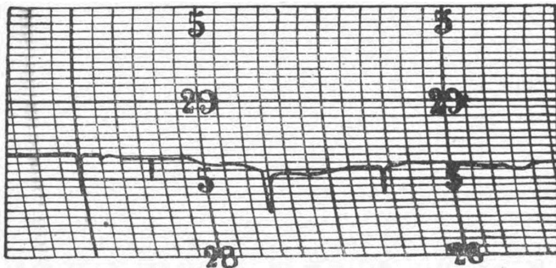
**Figure 4** - Changes in water level (at a point about 40-ft (12-m) deep and 140 ft (43 m) from train tracks) induced by moving trains as measured by a float attached to a lever arm with a pen that rested on a vertically oriented cylinder which rotated with time at the top of the well to record a rise in water level as downward motion of the pen (King, 1892).
