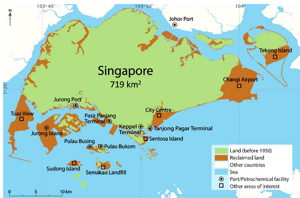
Figure 81 - Map of Singapore showing the amount of land reclaimed since 1950 (modified after Wells et al., 2019).
