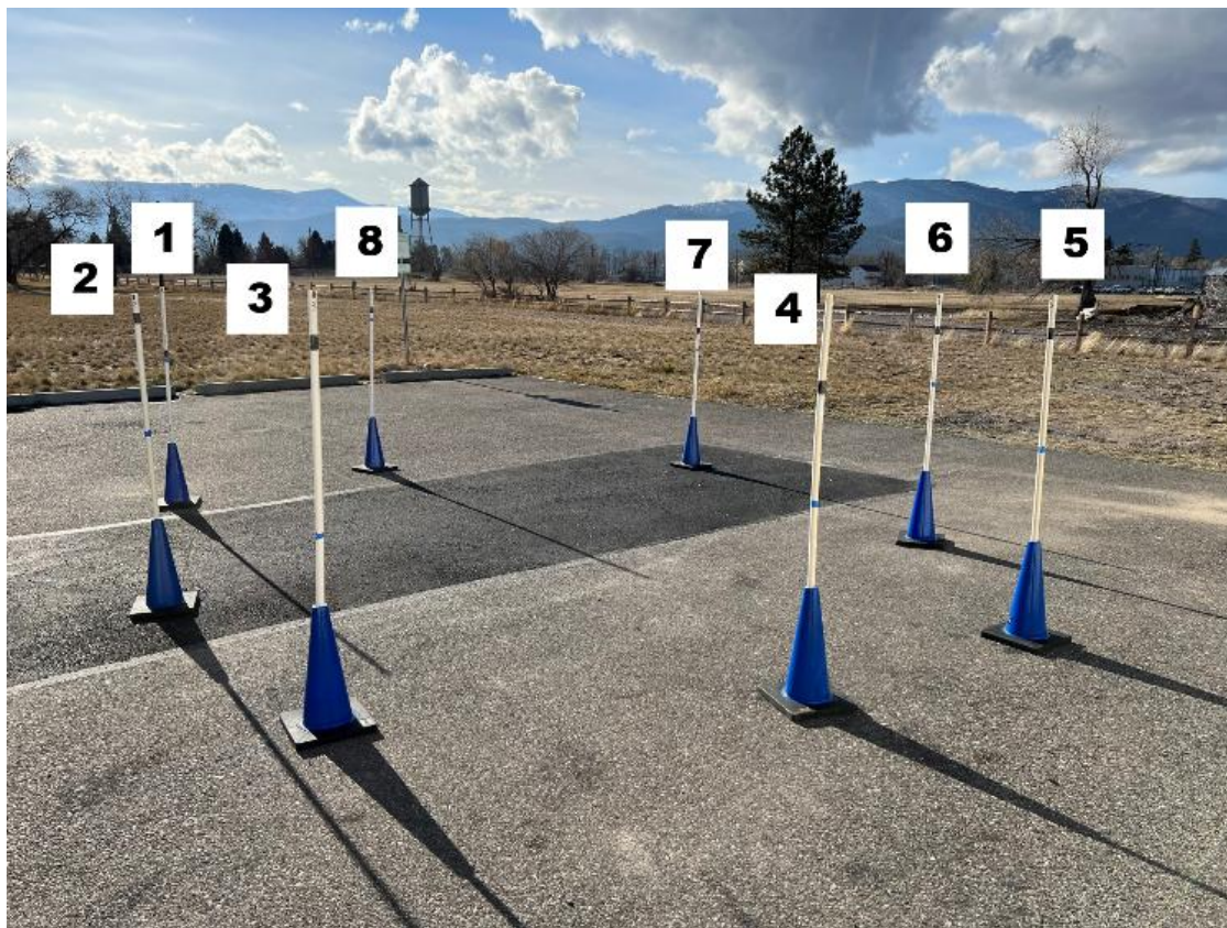
Figure 30 - Wells supported using small traffic cones. Well numbers are shown in black next to each well.
