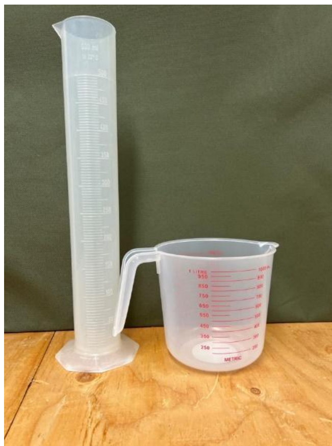
Figure 31 - Graduated cylinder and measuring cup used to fill model wells with water.
