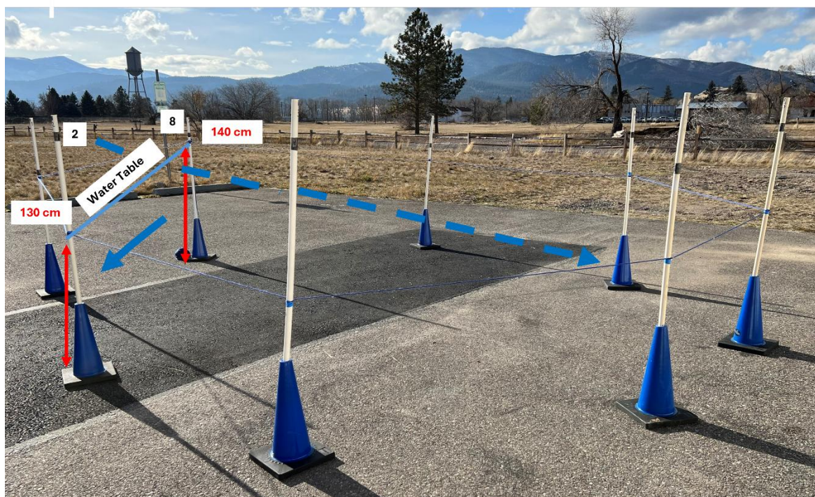
Figure 22 - An interpreted water table slope and direction of groundwater flow when only two wells are available, wells 2 and 8. Blue tape shows the water levels in the wells. The red arrows represent the water level elevations above the parking lot datum (head in red letters). Interpreted groundwater flow is from high head to low head (blue arrow). However, as the wells are not located along a groundwater flow line (dashed blue arrow), which can only be known by using at least three wells positioned in a triangle, the illustrated slope does not represent conditions in the three-dimensional system. When all head data are interpreted the shape of the water table shows groundwater flow goes from left to the right (dashed blue arrow).
