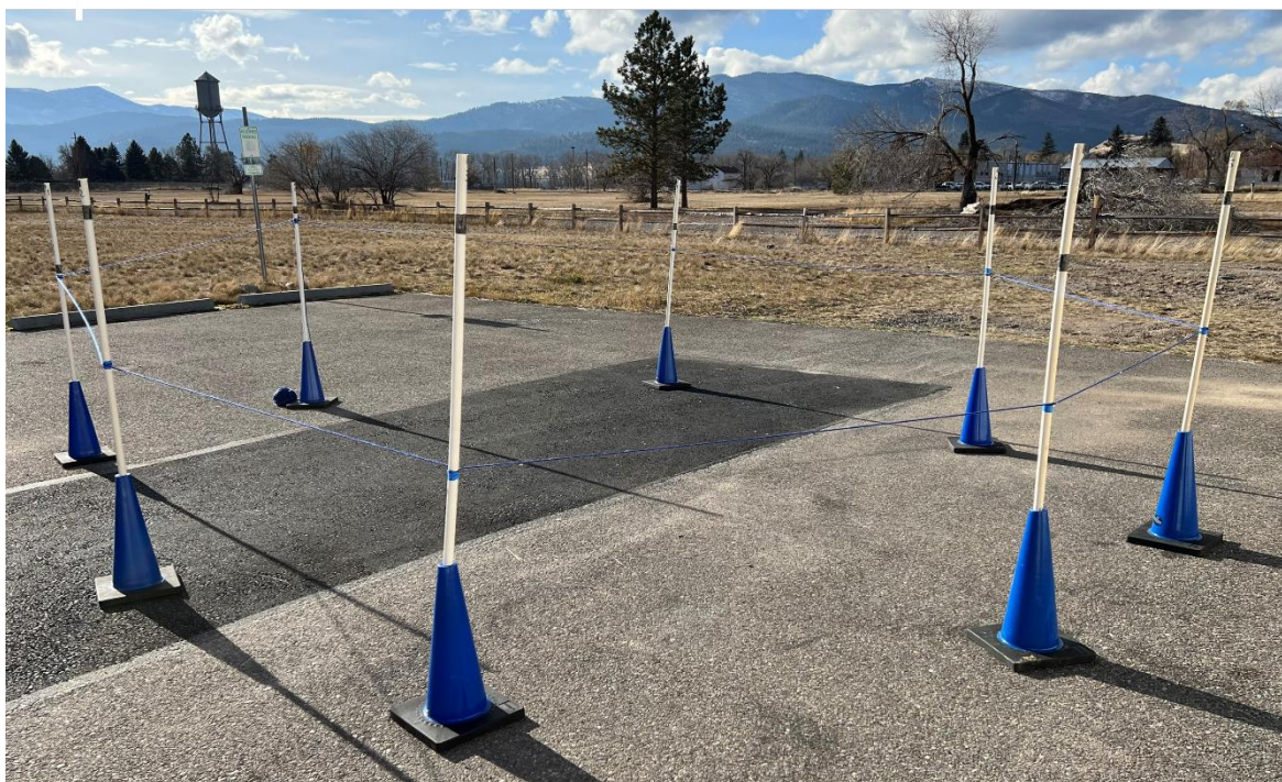
Figure 17 - Outdoor model with water levels representing the water table marked with blue tape. The three-dimensional water table surface has been outlined with blue yarn. The darker green-gray tape near the top of the casings was used to indicate the land surface position in this example.
