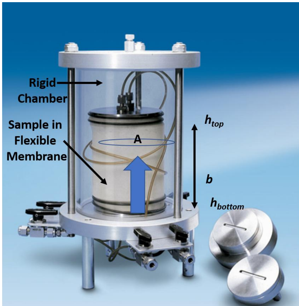
Figure Box 9-2 - Triaxial permeability cell. Valves and tubes shown connect to a control panel that supplies water, pressurization, vacuum, as well as methods to control gradients and measure flow rates. Water in the sample moves from the bottom to the top of the cell. A is the sample cross sectional area. The pressurized water in the rigid triaxial cell remains constant after being set by the user. The gradient is computed by subtracting the head at the top of the cell ( h_{top} , lower) from the head at the bottom of the cell ( h_{bottom} , higher), and dividing by the sample thickness, b . K_v is calculated after the flow rate reaches steady state (photograph modified from https://www.geo-con.com.au/product/permeability-cells/ ).
