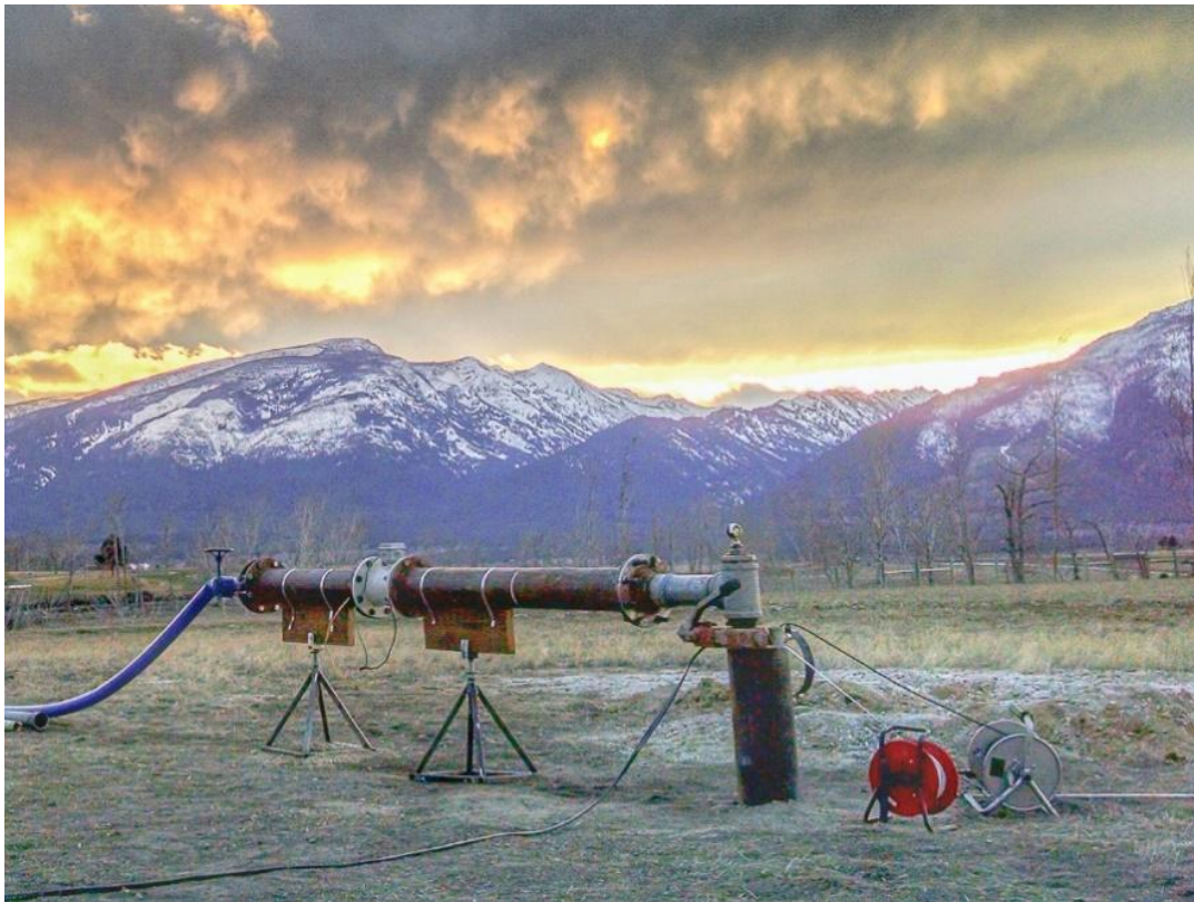
This photograph shows a pumping test being conducted in an unconfined sand and gravel aquifer in the Bitterroot valley, Western Montana, USA. The photograph is used with permission from Montana Bureau of Mines and Geology (2023).
