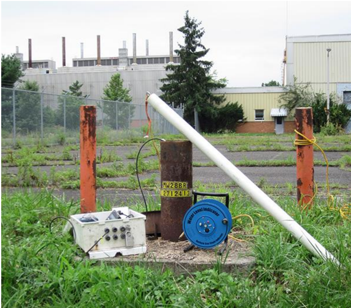
This photograph shows a solid weighted slug (capped white PVC pipe), pressure transducer recording box, and an electric tape used to conduct slug tests at the Naval Air Warfare Center in New Jersey, USA (USGS, 2014).
