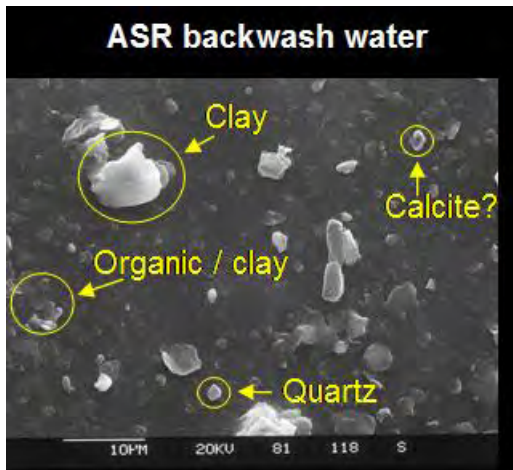
Figure 8 SEM micrographs showing particles in backwash water from ASR well on 10 Dec. 1999
