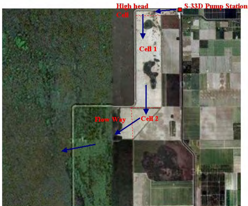
Figure 2. S-332D Basin with flow diagram and features (not to scale)
