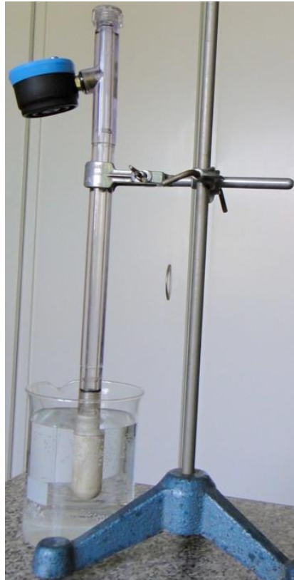
Figure 20 - A tensiometer, of which the porous cup would be placed in the soil with the pressure gauge exposed at the soil surface (image from the Czech University of Life Sciences Prague website). http://hydropedologie.agrobiologie.cz/images/tenzometr/tenz-foto03.jpg .
