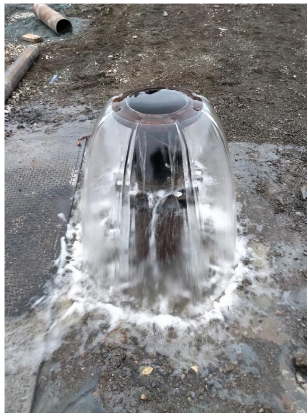
Figure 32 - Photograph of a flowing well (courtesy Jim Fyfe, Fyfe's Well Drilling). The well is flowing because the elevation of the potentiometric surface, or pressure head, in the zone where the well is screened is above the well head elevation.
