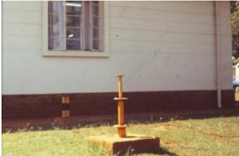
Figure 56 - Telescopic benchmark anchored in rock, and two higher elevated horizons (Photograph Wolmarans, 1984).
