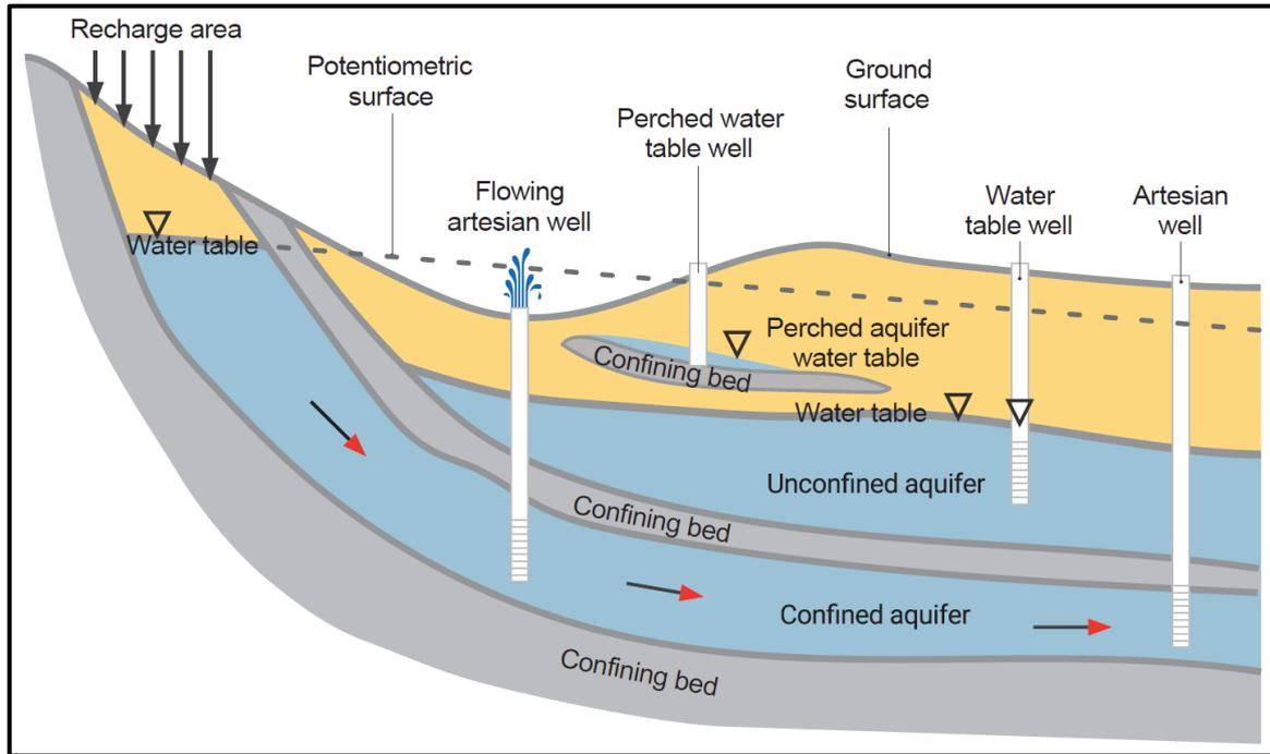
**Figure 2** - A commonly used but potentially misleading plot showing three types of aquifers and three types of wells, including a flowing artesian well tapping the confined aquifer (modified from United Nations, 2022).
