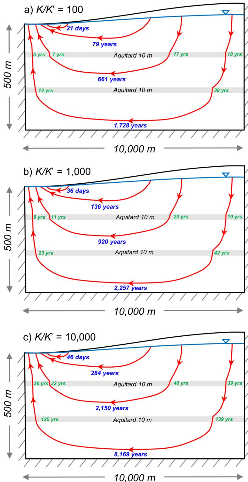
**Figure 32** - The time scales of groundwater circulation from recharge to discharge areas along different flow paths (numbers in blue) under three different, aquifer-aquitard hydraulic conductivity contrasts ( $K/K'$ ). The green numbers indicate the time required for the flow line to reach the other side of the aquitard [conversions: 10 m = 32.81 ft; 500 m = 1,650 ft; 10,000 m = 32,800 ft].
