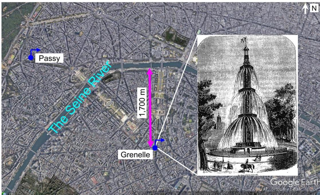
**Figure 8** - The location of the Grenelle Well and the Passy Well, Paris, France. The inset is an illustration from 1860 showing the Grenelle Well functioning as a fountain (reproduced from Botham, 2021; 1,700 m  $\cong$  1 miles).
