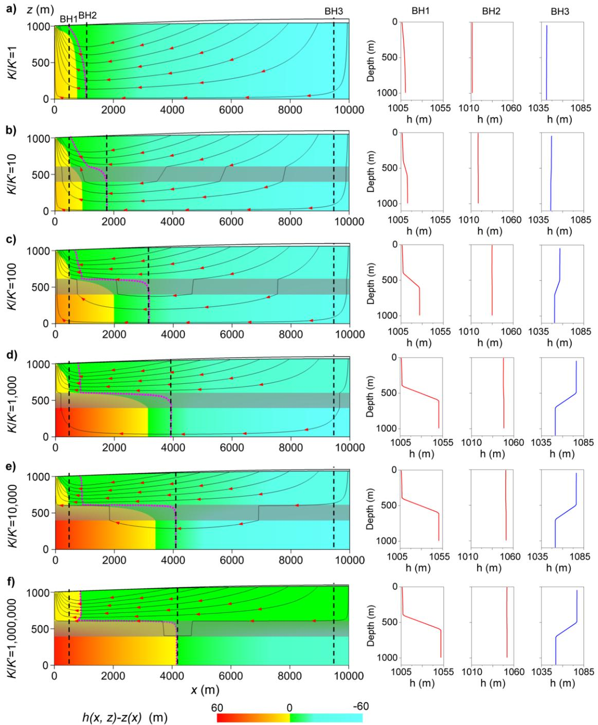
**Figure 30** - The distributions of flow paths and zones where head exceeds land surface in basin cross sections along with vertical profiles of hydraulic head in three hypothetical boreholes under six aquifer-aquitard hydraulic conductivity contrasts ( $K/K$ ).
