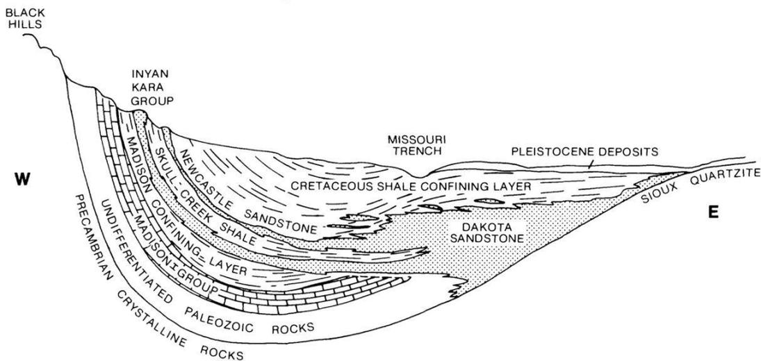
Figure 16 - West to east cross section showing the Dakota aquifer system (reproduced from Bredehoeft et al., 1983).
