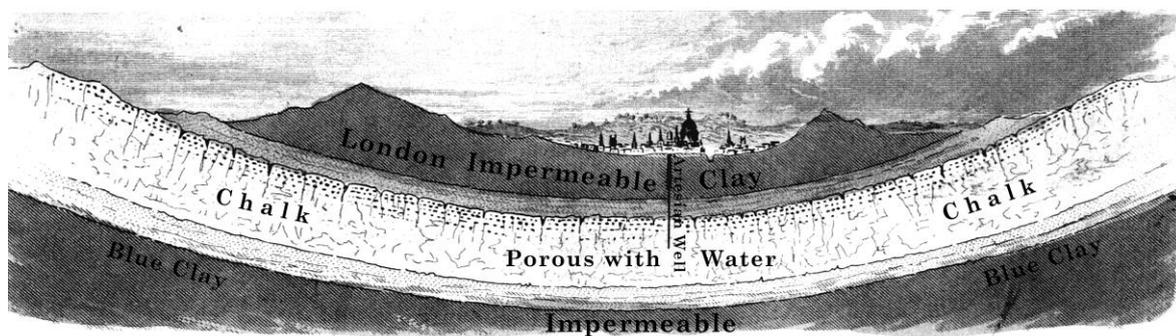
*The rain falling upon the porous Chalk, descends and accumulates in its lowest parts being retained by the impermeable Clay above and below. If the upper Clay is penetrated by an Artesian Well, the water will rise in the bore to its corresponding level in the Chalk.*
