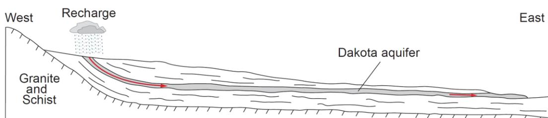
**Figure 24** - The profile of the Dakota, USA, confined aquifer and its confined flow bounded by aquitards (modified from Fetter, 2001). The red lines with arrows represent the direction of confined flow.
