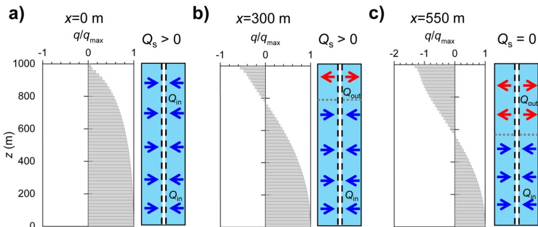
**Figure 45** - Vertical variations of dimensionless radial discharge rate of fully penetrating flowing wells installed at different distances away from the valley. The cases (a) and (b) are flowing wells, whereas the case (c) is a non-flowing well.
