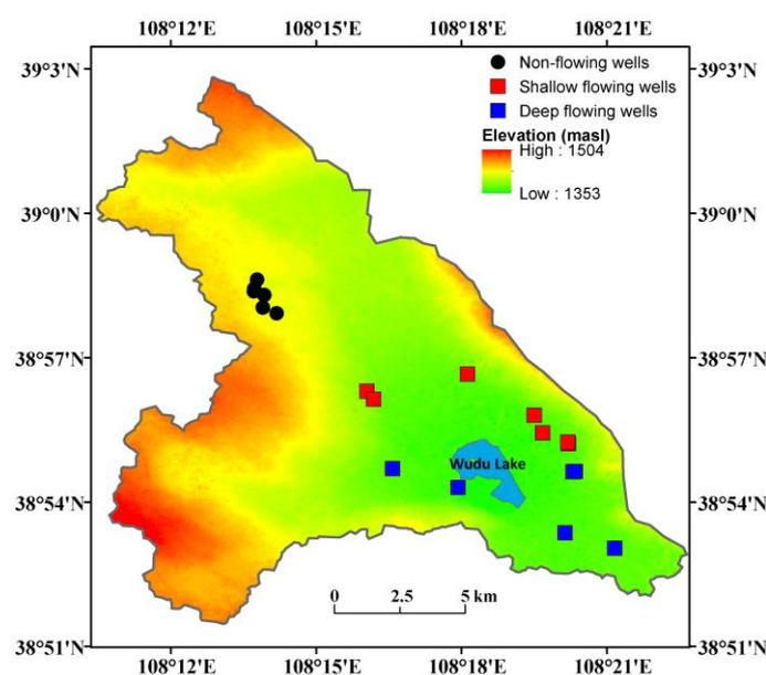
**Figure 23** - Locations of non-flowing wells in topographic highs and flowing wells in topographic lows in the Wudu Lake catchment, Ordos Plateau, China (modified from Ji et al., 2022) [1,353 masl = 4,438 ft above sea level (fasl); 1,504 masl = 4,934 fasl].
