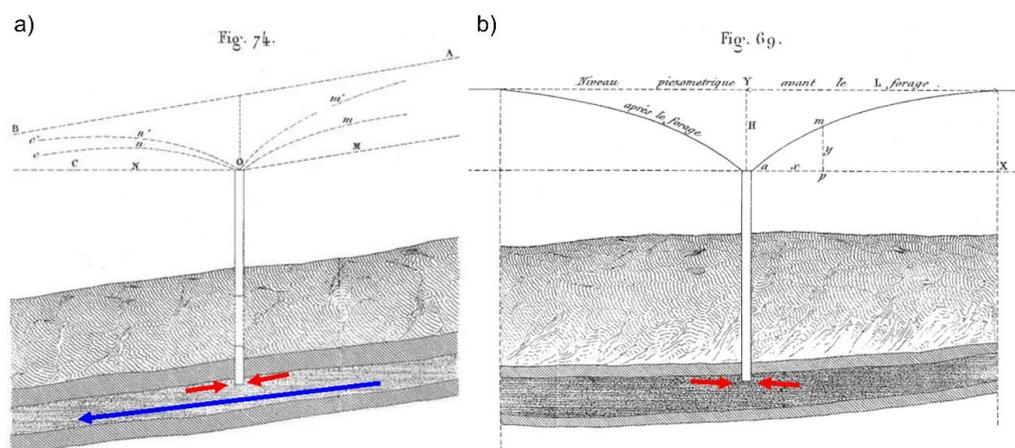
**Figure 34** - Diagrams from Dupuit (1863) showing radial flow toward a flowing well penetrating a confined aquifer, which caused head loss with a cone of depression in the potentiometric level (*niveau piézométrique*; transl.: new piezometric). The regional hydraulic gradient is considered in a) and neglected in b). The red arrows in (a) and (b) are added to show the direction of radial flow. The blue arrow in (a) is added to show the direction of regional flow.
