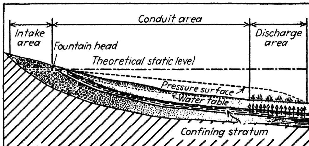
**FIG. 133.**—Artesian conditions in stratiform aquifer.
