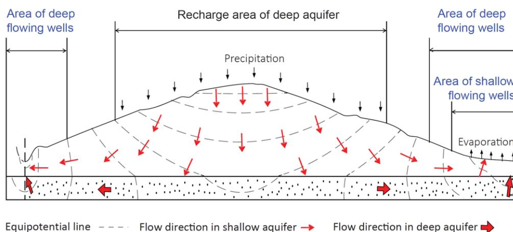
**Figure 21** - The Prairies Profile showing topographically driven flow systems in a heterogeneous basin with a higher permeability layer in the bottom (modified from Meyboom, 1962). The solid line represents the topography.
