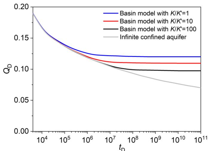
**Figure 40** - Dimensionless discharge rate ( $Q_D$ ) of the flowing well tapping the semi-confined aquifer versus dimensionless time ( $t_D$ ) in the three-layer basin (modified from Zhang et al., 2022). The gray line represents that of a flowing well tapping an infinite confined aquifer. Steady state flow is greater when more water can penetrate the aquitard (i.e., when  $K/K'$  is smaller).
