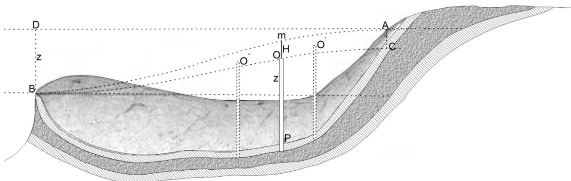
**Figure 10** - Flowing wells (O, O', and O'') tapping the confined aquifer in the topographic lows of the Paris Basin. Also shown are the potentiometric surfaces (AB and CB) at two states (from Dupuit, 1863; modified from Ritzi & Bobec, 2008).
