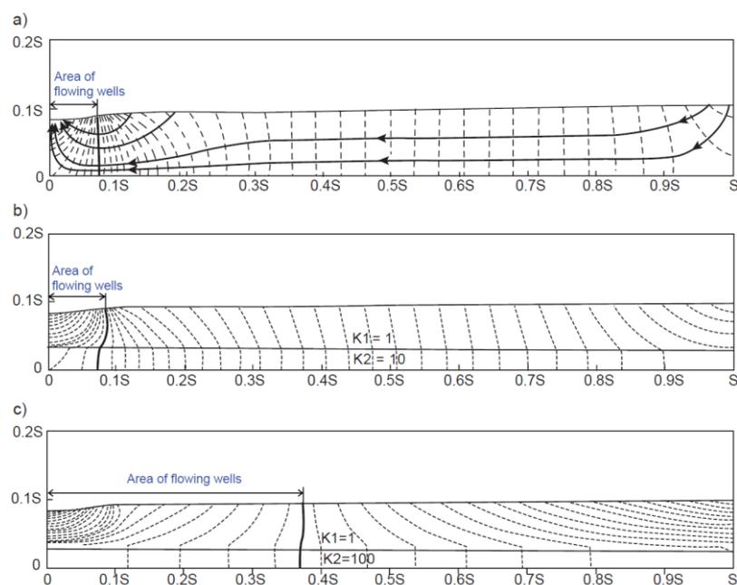
**Figure 28** - a) Distributions of equipotential lines, streamlines, and area with flowing wells in a homogeneous basin. b) and c) The enlargement of area of flowing wells in two-layer basins with different  $K_2$  (modified from Freeze & Witherspoon, 1967). As  $K_2$  increases, the area of flowing wells expands significantly.
