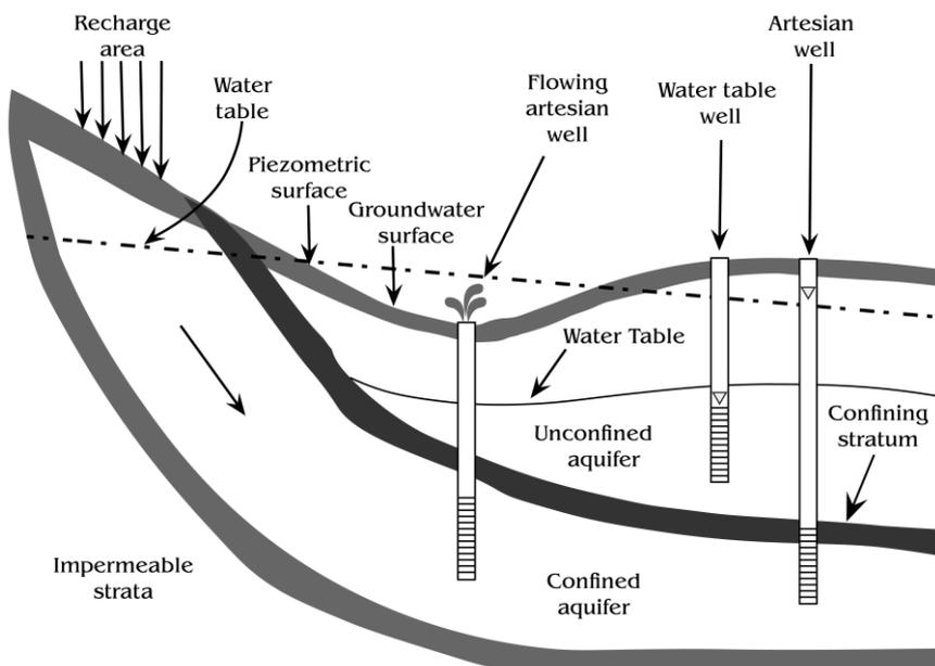
**Figure 26** - A schematic showing unconfined and confined aquifers, with a flowing well and an artesian well tapping the confined aquifer (modified from Todd, 1959).
