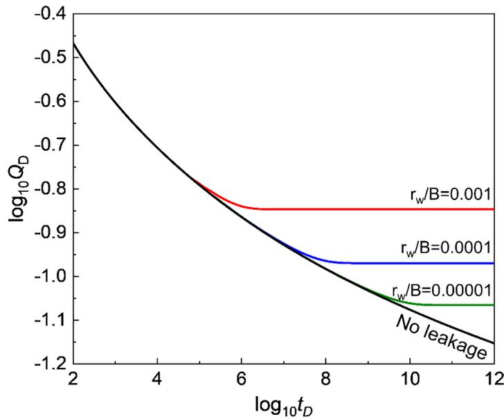
**Figure 38** - Relationship between  $Q(t_D, r_w/B)$  and  $t_D$  for a range of  $r_w/B$ . The flattening of the drawdown at the later time indicates steady-state has been reached because of leakage. Note that the well radius,  $r_w$ , is fixed but the leakage factor,  $B$ , is not fixed. As  $r_w/B$  increases, steady-state occurs sooner due to the decreasing  $B$ .
