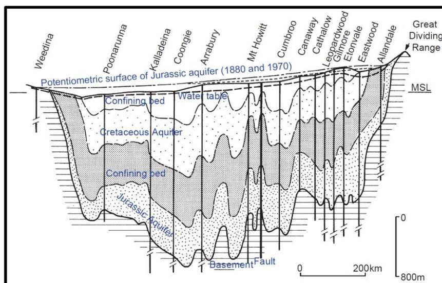
**Figure 20** - Simplified cross section of the Great Artesian Basin, Australia, showing the major aquifers and confining units (modified from Habermehl 1980) [200 km  $\cong$  124 miles, 800 m  $\cong$  2,625 ft].
