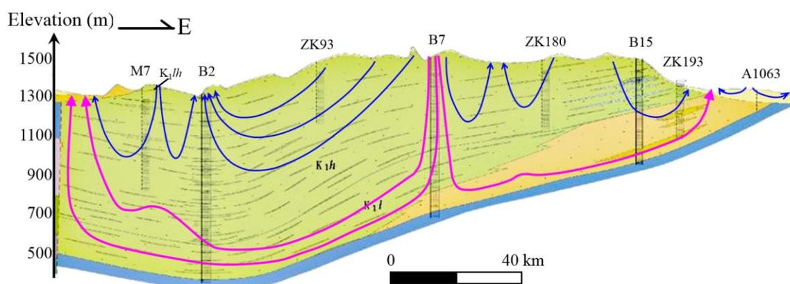
**Figure 22** - A geological cross section in the Ordos Plateau, China, showing topographically controlled groundwater flow in the thick Cretaceous sandstone aquifer with no continuous aquitards (modified from Hou et al., 2008) [conversions: 40 km = 25 miles; 500 m = 1,640 ft; 1,500 m = 4,921 ft].
