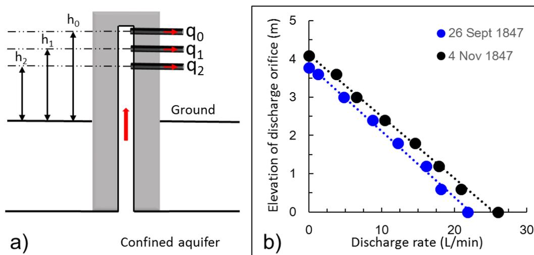
**Figure 33** - a) A schematic of a device with three discharge orifices for measuring discharge rate (only one discharge orifice is open during measurement).  $h_0$ ,  $h_1$ , and  $h_2$  are elevations of the three discharge orifices, while  $q_0$ ,  $q_1$  and  $q_2$  are discharge rates at each orifice; b) Changes in discharge rate with elevation of discharge orifice of a flowing well above the ground surface (data from Darcy, 1856).
