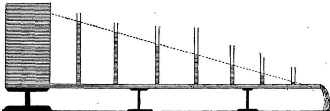
Figure 18 - An apparatus used to illustrate the flow pattern in a purely confined aquifer (reproduced from Darton, 1905). The left reservoir represents groundwater in the recharge area, which flows toward and discharges on the right side. The vertical pipes represent piezometers, and the dashed line represents the potentiometric surface with linearly decreasing hydraulic head.
