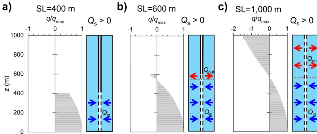
**Figure 44** - Vertical variations of dimensionless flow rate in flowing wells with different screen lengths (SL) in a homogeneous basin. a) A flowing well with  $Q_{in} > Q_{out} = 0$ ; b) a flowing well with  $Q_{in} > Q_{out} > 0$  and c) a flowing well with  $Q_{in} > Q_{out} > 0$ . In all the cases shown  $Q_s > 0$  because  $Q_{in}$  exceeds  $Q_{out}$ .
