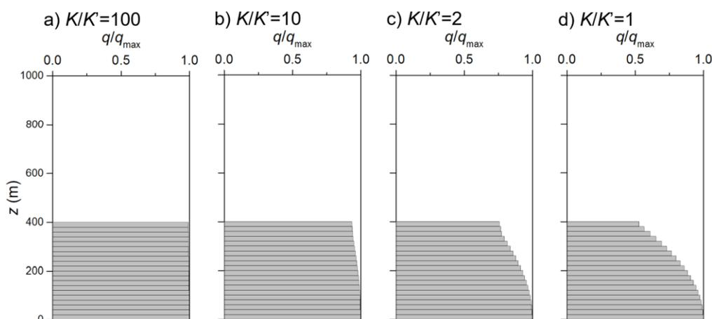
**Figure 43** - Vertical variation of dimensionless flow rate in a flowing well tapping the deep part of a basin (located at  $x = 400$  m, 1,312 ft) with different  $K/K'$ . As  $K'$  increases, the trend of increasing flow rate with depth becomes more significant.
