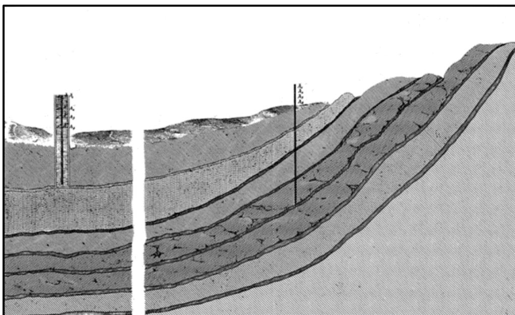
**Figure 9** - Stratigraphy and structural geology of the Paris Basin (from Darcy, 1856; reproduced from Ritzi & Bobec, 2008). The well on the left (representing the famous Grenelle Artesian Well) taps a Cretaceous sandstone (the *Greensand* in Darcy's time) that is interstratified with thicker chalk strata.
