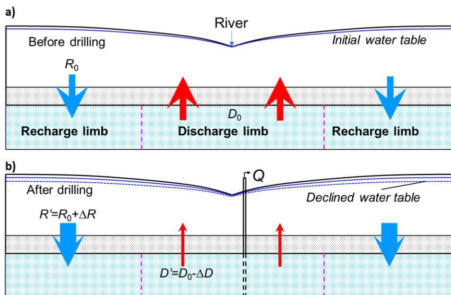
**Figure 42** - A schematic representation of inter-aquifer leakage in the basin before a) and after b) installing a flowing well near the river (modified from Zhang et al., 2022). The larger downward blue arrows in (b) represent increased recharge, and the smaller upward red arrows in (b) represent decreased discharge. The flow field before installing a flowing well can be found in Figure 30.
