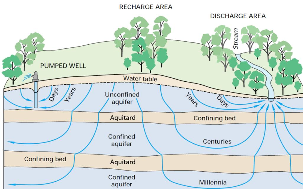
**Figure 31** - The pattern and time scales of groundwater flow from recharge to discharge areas in a five-layer basin described by Heath (1983; modified from Winter et al., 1998).
