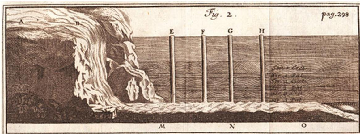
**Figure 4** - Bernardino Ramazzini's conceptual drawing shows the cause of flowing wells in a confined aquifer (reproduced from Duffy, 2017).
