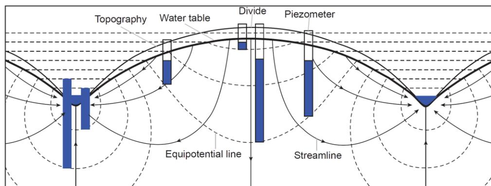
**Figure 27** - The flow net of groundwater flow between two streams obtained by Hubbert (1940) (modified from Fetter, 1994). The blue bars represent pressure head in selected piezometers.
