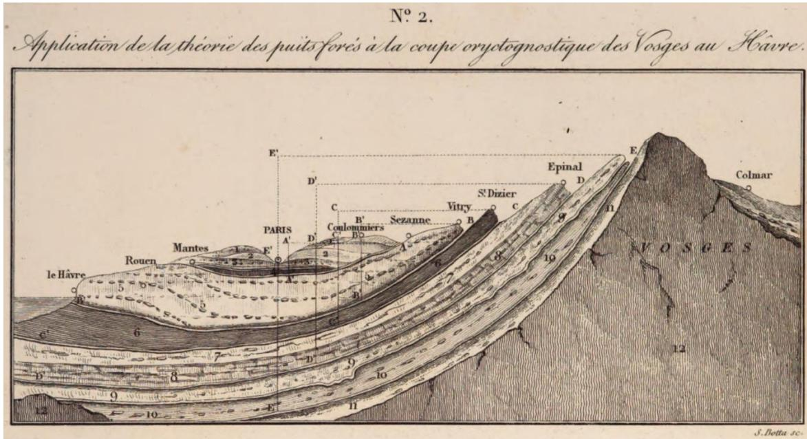
**Figure 7** - A cross section showing the geology and the potentiometric surfaces in the Paris Basin. A limitation is the neglect of head loss through the conduits (reproduced from Héricart de Thury, 1829).
