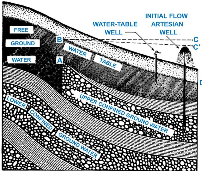
**Figure 25** - A schematic showing free groundwater, confined groundwater and a flowing well (reproduced from Tolman, 1937). The label "A" indicates the upper edge of the upper confined aquifer; BC and BC' are the theoretical and actual static levels of the upper confined aquifer; BD is the water table.
