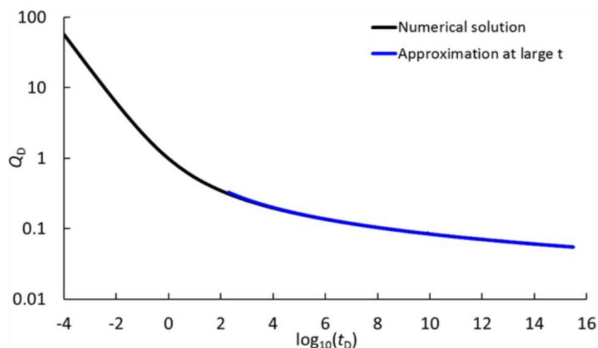
**Figure 36** - The curve of dimensionless discharge rate  $Q_D$  versus the dimensionless time  $t_D$ .
