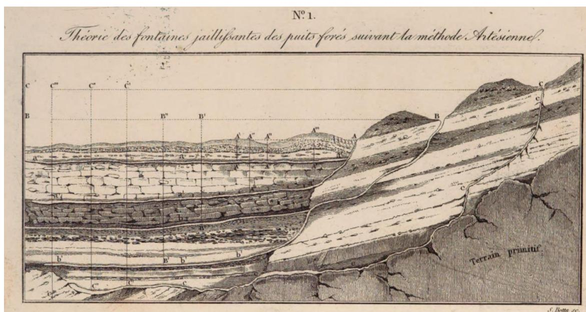
**Figure 6** - A schematic plot showing potentiometric surfaces of three different conduits (starting from A, B, and C) between formations. A limitation is the neglect of head loss through the conduits (reproduced from Héricart de Thury, 1829).
