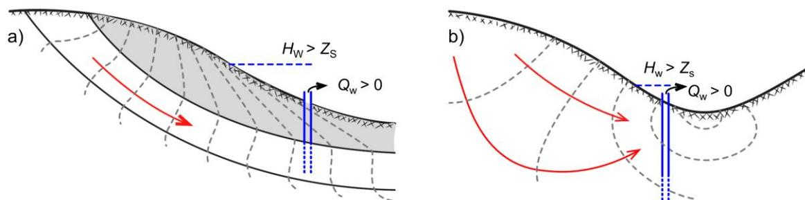
**Figure 3** - Cross sections showing two endmember conditions of flowing wells: a) a geologically controlled flowing well in the confined aquifer of a basin; b) a topographically controlled flowing well in a homogeneous basin (modified from Freeze & Cherry, 1979).  $Q_w$  represents the discharge rate of the flowing well,  $H_w$  represents the hydraulic head near the flowing well, and  $Z_s$  represents the elevation of the land surface near the flowing well.
