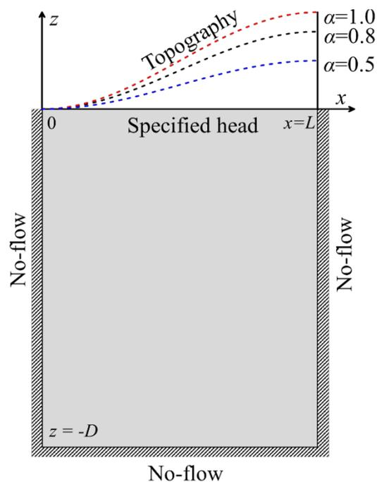
The geometry of a unit basin with a length of  $L$ , depth of  $|D|$ .
