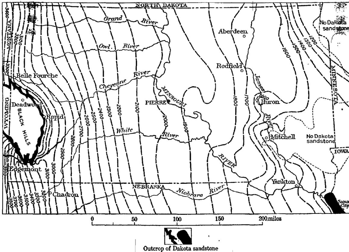
Figure 17 - Contours of hydraulic head showing the hydraulic gradient of the Dakota sandstone aquifer in South Dakota (reproduced from Darton, 1909; 50 miles = 80.47 km).
