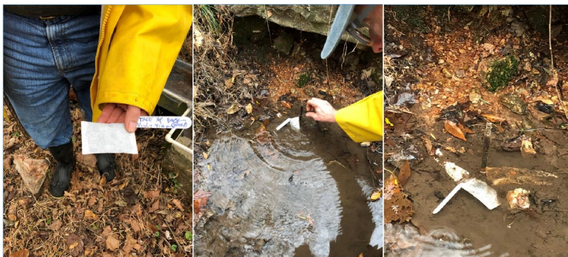
Figure 52 - Photographs of J. Van Brahana setting a bug (dye absorbent material in a flow through mesh bag) at Tree Spring at the Savoy Experimental Watershed, Arkansas, USA. The bug is fixed in place (usually for days or weeks) to determine if dye passes that location, but the exact time of arrival cannot be determined. Photograph by Kuniansky (2017)
