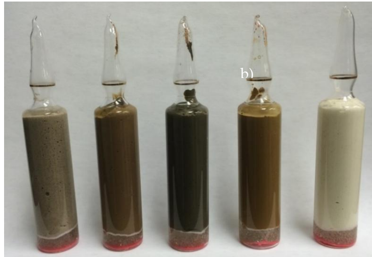
Figure Box-6-2 - Ampule vial setup with field soils and lab-grade soil.
