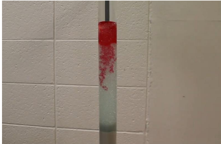
Figure 45 - Downward Migration of DNAPL: an animated version of this is shown in this video .
