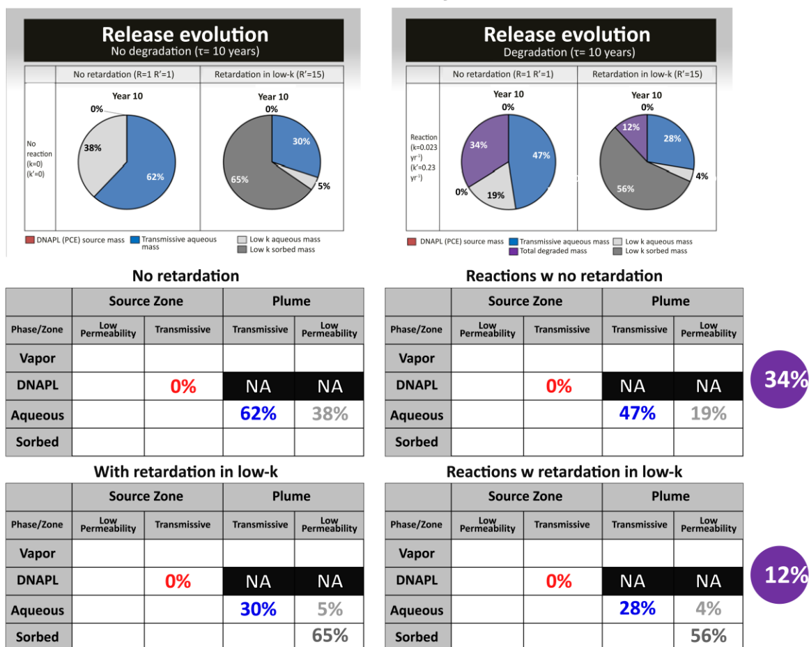
Figure 94 - Distribution of contaminants in the 14C model and losses due to reactions at t = 10 years for the conceptual model shown in Figure 87 and parameterized as indicated in Table 4 (adapted from Wahlberg, 2013).
