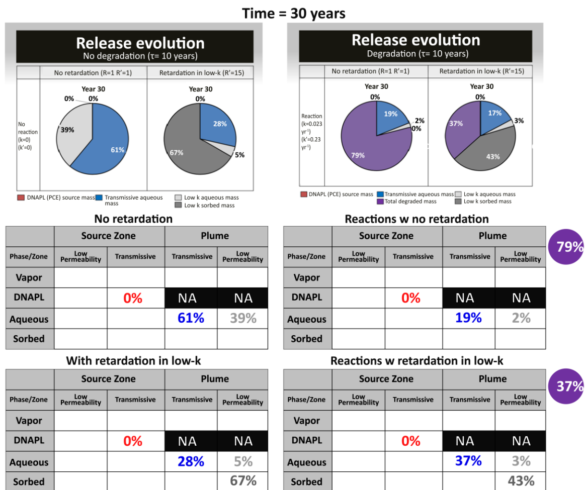
Figure 96 - Distribution of contaminants in the 14C model and losses due to reactions at t = 30 years for the conceptual model shown in Figure 87 and parameterized as indicated in Table 4 (adapted from Wahlberg, 2013).
