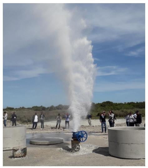
**Figure 46 -** Artesian flow from a future production borehole on the Coega Fault, tapping the Table Mountain Group, Eastern Cape, South Africa. Stable isotope information can help manage such large, deep groundwater reserves sustainably.
