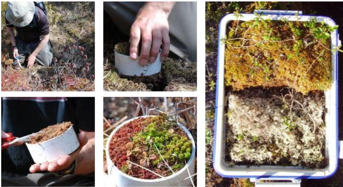
**Figure 23** - Sampling of the upper layer of bog peat using a 10 cm diameter, 5 cm tall PVC ring, using a knife and scissors. Lower layers can be sampled sequentially. Larger samples can be cut with serrated knives or a handsaw; storage in a rigid cooler or container is advised. (Photographs by J. Price, C. McCarter, and W. Quinton)
