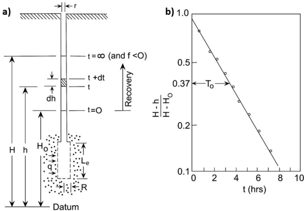
a) Identification of values  $H$ ,  $H_0$ , and  $h$ , at different times ( $t$ ), as well as  $r$ ,  $R$ , and  $L_e$ ; b)  $K_{sat}$  is determined by the rate of recovery, which is portrayed here on a log-linear plot, from which  $T_o$  is estimated from a point on the line corresponding to  $(H-h)/(H-H_0) = 0.37$ . Diagram from Freeze and Cherry (1979).
