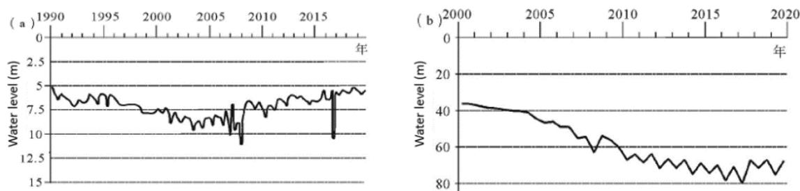
**Figure 15** - Groundwater levels in typical monitoring wells in the shallow aquifer, North China Plain (after Yang et al, 2021)
