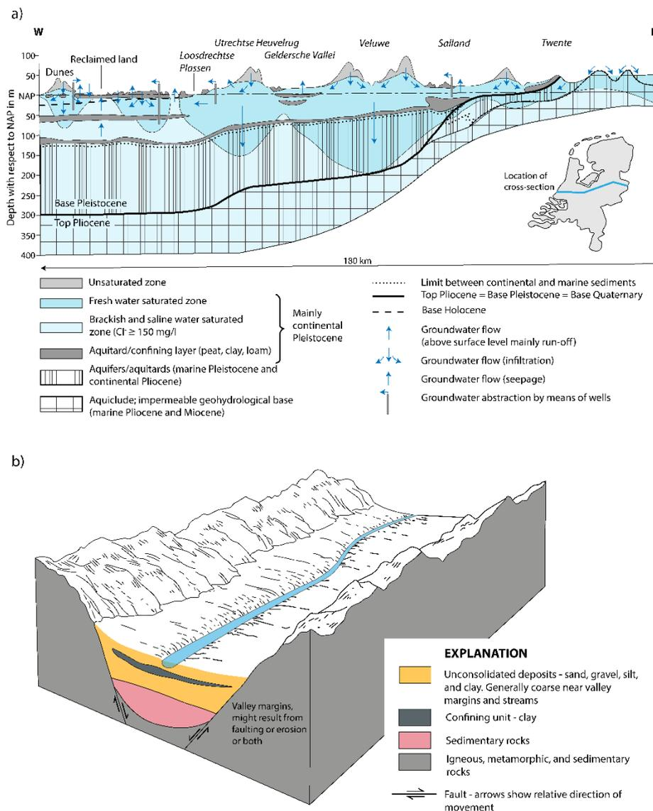
**Figure 3** - Two examples of sand and gravel aquifers in different geological settings: a) a hydrogeological cross-section through The Netherlands showing a multi-layer aquifer system in a subsiding geological basin, bordered at its western margin by the North Sea (Dufour, 2000); and, b) a conceptualization of a basin-fill aquifer (USGS, 2000).
