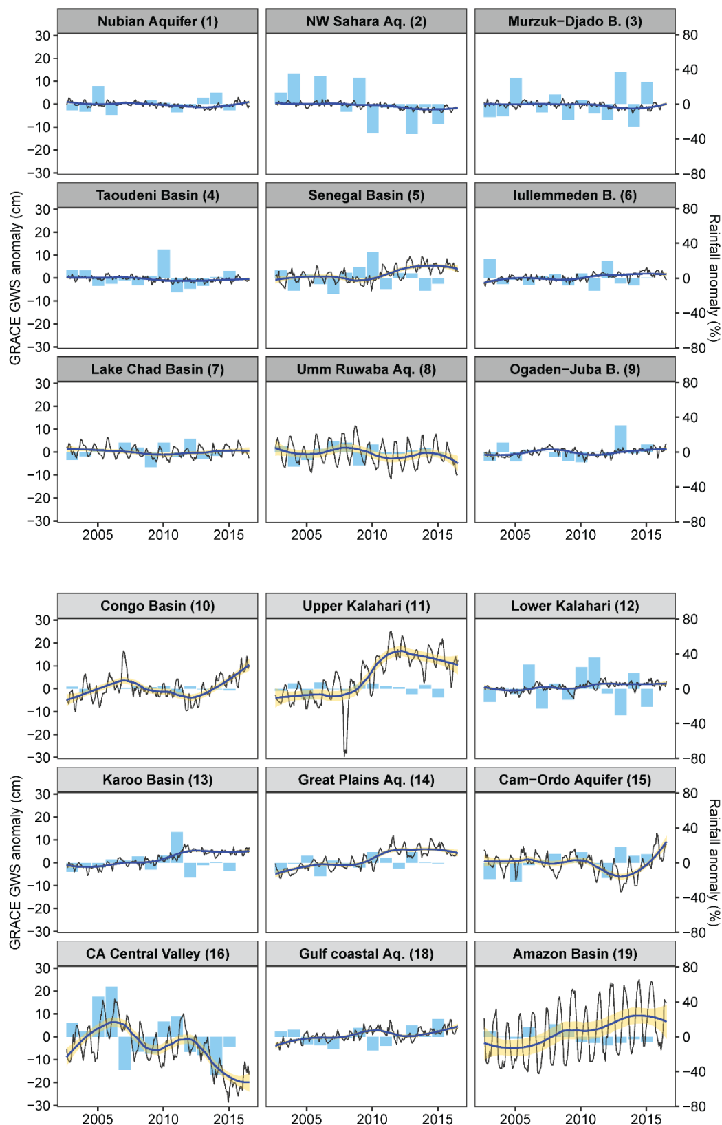
Figure 21 - Monthly time series of groundwater storage anomalies derived from GRACE for the mega aquifers 1 through 19 (except number 16), August 2002 to July 2016. The ensemble GRACE-derived \Delta GWS (in black) is fitted with a non-linear trend curve (the area shaded in semi-transparent gold shows the 95 percent confidence interval) and annual precipitation anomalies (i.e., percentage deviation from the mean precipitation for the period of 1901 to 2016) are shown as bars (Adapted from Shamsudduha and Taylor, 2020).
