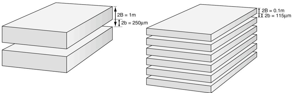
Figure 1.3. Two different fractured rock systems with identical hydraulic conductivities ( $10^{-5} \text{ m s}^{-1}$ ). a) aquifer comprising identical planar, parallel fractures, with fracture aperture of  $250 \mu\text{m}$  and fracture spacing of  $1 \text{ m}$ , b) aquifer comprising identical planar, parallel fractures, with fracture aperture of  $115 \mu\text{m}$ , and fracture spacing of  $0.1 \text{ m}$ .
