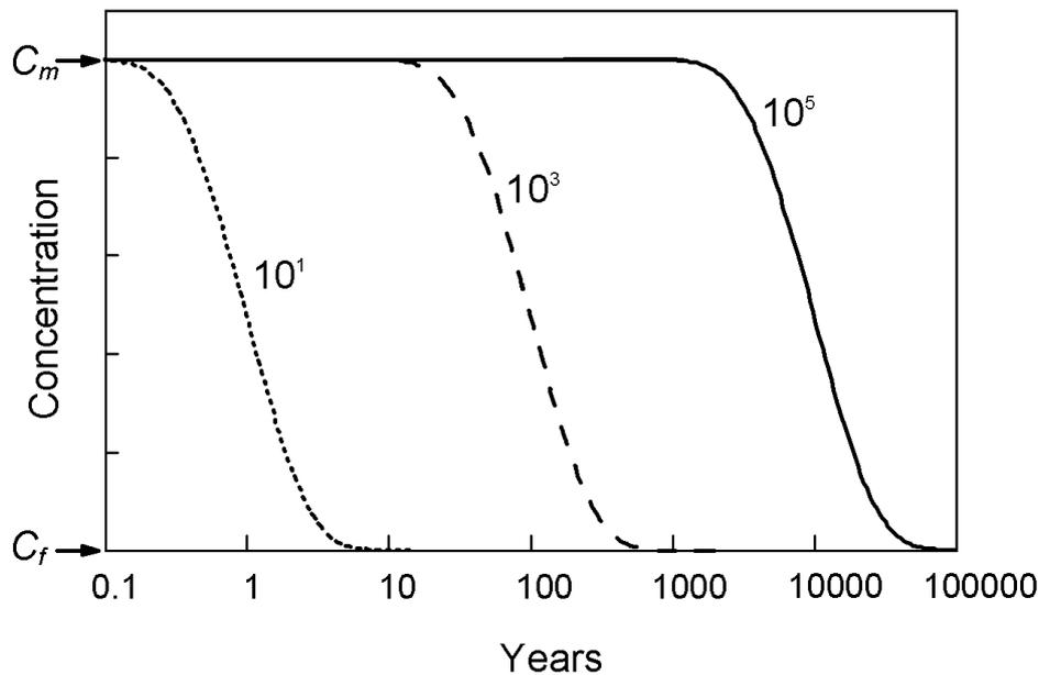
Figure 5.13. Time for solutes to diffuse from the aquifer matrix into the fractures. The decrease in solute concentration in the aquifer matrix mid-way between the fractures is plotted as a function of time. Numerals indicate values of  $(2B)^2/D = 10, 1000, \text{ and } 10^5$  years.
