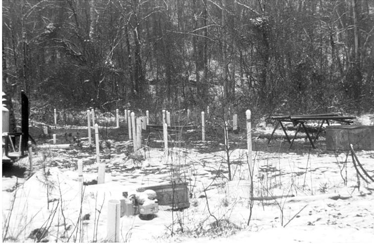
Figure 5.9. Part of the bore network for the natural gradient tracer test in fractured shale, West Bear Creek Watershed, Oak Ridge, Tennessee.
