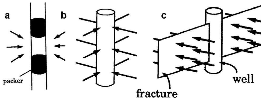
Figure 4.5. Contrasting models of groundwater flow to a well, that are used for interpreting single well hydraulic tests. (a) Flow to a short test interval in a borehole that approximates spherical geometry (interval length  $\approx$  borehole radius); (b) Radial flow to a cylinder; and (c) Linear flow to a well that intersects a highly transmissive vertical fracture. (From NRC, 1996.)
