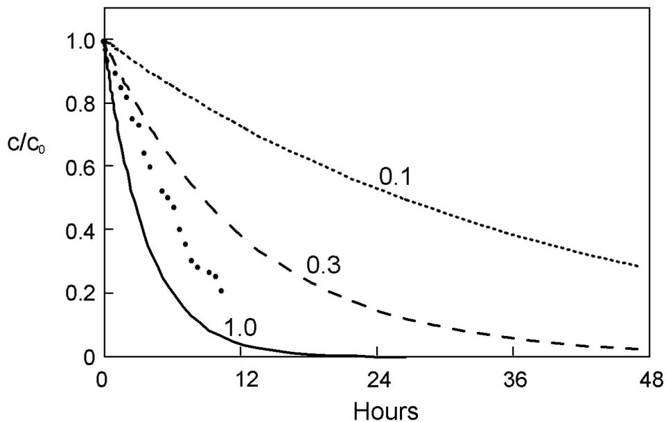
Figure 5.3. Theoretical concentration versus time curves for point dilution tests in a well of radius  $r = 0.1 \text{ m}$ , and where the added tracer is not naturally present within the groundwater ( $c'=0$ ). Flow rates of  $q = 0.1, 0.3$  and  $1.0 \text{ m day}^{-1}$  are compared. Circles denote results of a point dilution test in fractured rock in Maine, USA (Sidle & Lee, 1995).
