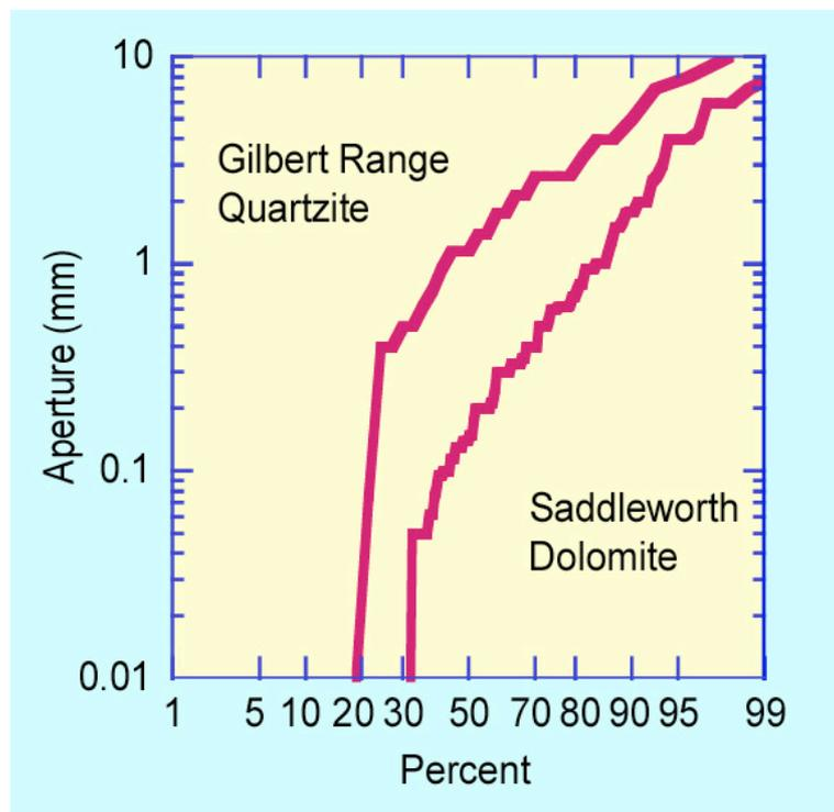
Figure 3.7. Distribution of fracture apertures measured with a feeler gauge on exposures of the Gilbert Range Quartzite and Saddleworth Dolomite, Clare Valley, South Australia. The x-axis refers to the proportion of apertures that are less than the specified value. Thus, for example, in the Saddleworth Dolomite, 90% of fracture apertures are less than 2 mm. The distributions are truncated at the lower end, because of the inability to measure very small fractures. (From Love *et al.*, 2002).
