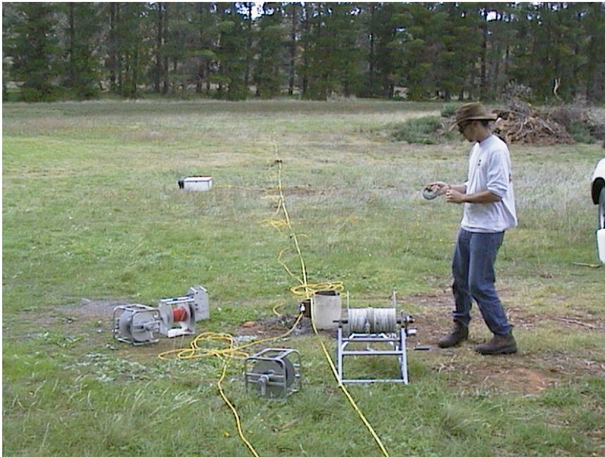
Figure 4.12. Carrying out an azimuthal resistivity survey, centred on a borehole, in the Clare Valley. Photo courtesy of Graham Heinson, University of Adelaide.
