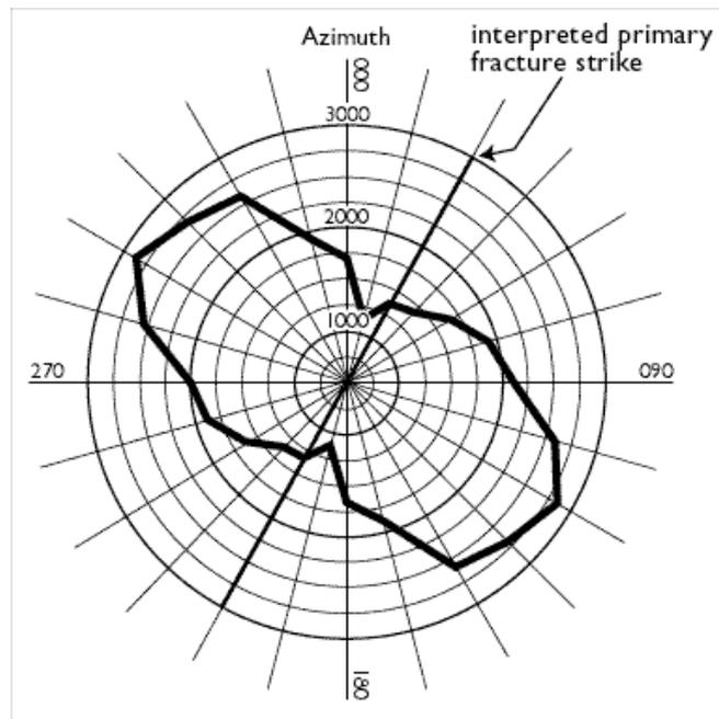
Figure 4.14. Square array resistivity data (ohm metres) from Mirror Lake, New Hampshire. The resistivity maxima occur at  $120^\circ$  and  $300^\circ$ , suggesting a primary fracture strike of  $30^\circ$ . (From Lane *et al.*, 1995.)
