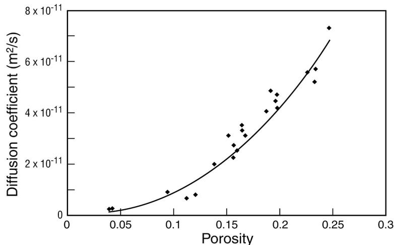
Figure 3.9. Relationship between solute diffusion coefficient for KBr and matrix porosity for core samples of Lincolnshire Limestone. (From Greswell *et al.*, 1998).
