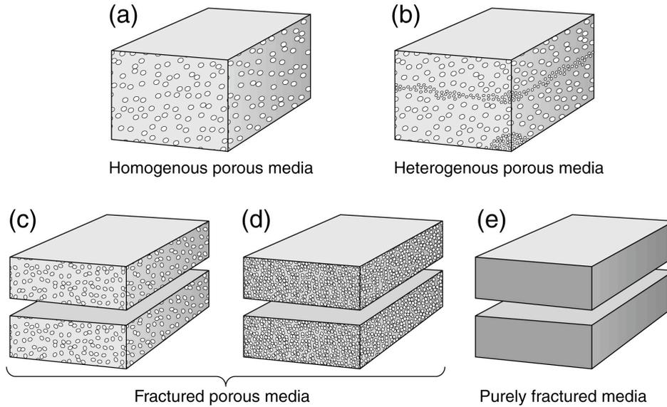
Figure 1.1. Classification of porous and fractured rocks: a) homogeneous porous media, b) heterogeneous porous media, c) fractured porous media with significant permeability in the aquifer matrix, d) fractured porous media with significant porosity, but negligible permeability in the aquifer matrix, e) purely fractured media, with zero porosity and zero permeability within the aquifer matrix.
