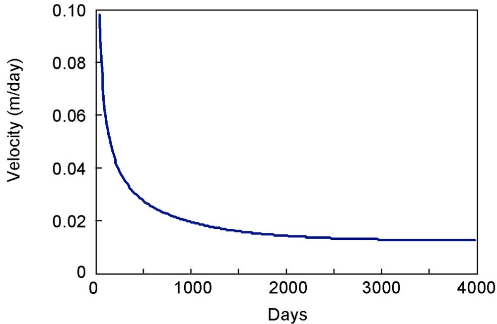
Figure 1.6. Apparent velocity of a tracer in fractured rock. Initially, the tracer velocity appears to decrease with time as solute diffuses into the rock matrix. At very late times, diffusion may result in equivalent tracer concentrations within the fractures and the aquifer matrix. When this occurs, the tracer velocity will not change with time. The curve shown is for  $V_w = 500$  m/year,  $\theta_m = 0.1$ ,  $B = 0.05$  m,  $b = 50$   $\mu\text{m}$ ,  $D = 10^{-5}$   $\text{m}^2/\text{yr}$ .
