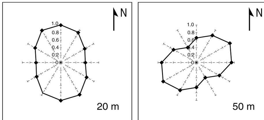
Figure 4.15. Normalised apparent resistivity polar plots for a Wenner array survey in the Clare Valley with electrode separations of 20 and 50 m. (After Wilson *et al.*, 2000.)
