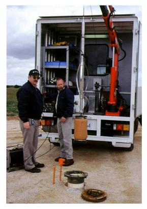
Figure 4.10. Preparing to carry out borehole flowmeter measurements. Photo courtesy of Paul Pavelic, CSIRO.
