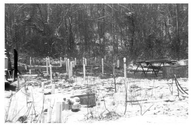
Figure 5.9. Part of the bore network for the natural gradient tracer test in fractured shale, West Bear Creek Watershed, Oak Ridge, Tennessee. Photograph courtesy of William Sanford, Colorado State University.
