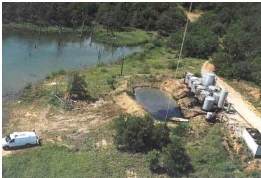
**Figure 58** - Aerial photograph of part of the OSPER B site showing the fluid tanks and the active brine pit near Skiatook Lake. Oil operations have caused the scarred and partially remediated area between the brine pit and the reservoir (photo courtesy of Ken Jewell, USEPA, Ada, Oklahoma; from Kharaka & Dorsey, 2005).
