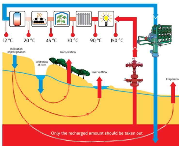
**Figure 33** - The scheme of an optimal geothermal cascade system to utilize the biggest heat amount. (modified after Szanyi et al., 2015)
