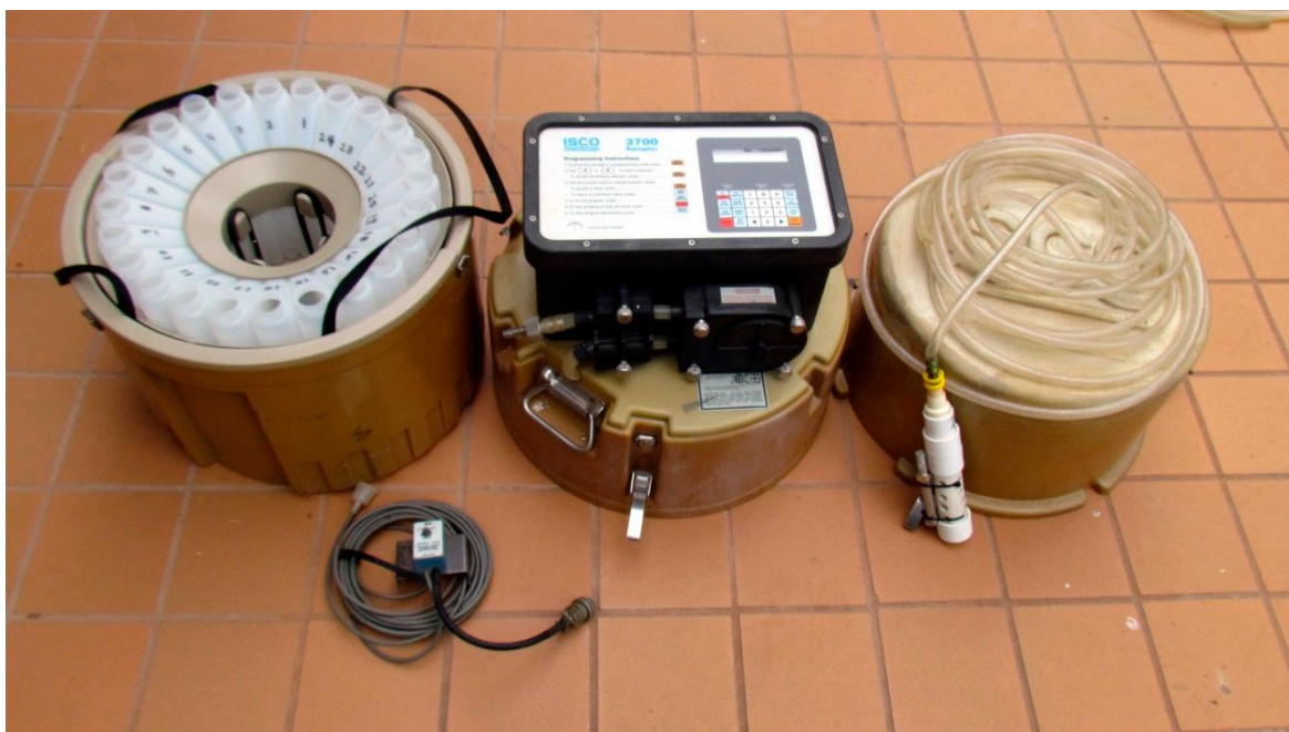
Figure 14 - Photo of ISCO 3700 programmable water sampler. The bottom portion of the sampler, shown on the left side of the figure, contains 24 numbered bottles. The middle portion controls programming, and the top portion, shown on the right side of the image, provides a weatherproof cover. Water intake is through the white tube and connected tubing. A storage battery to power the unit is not shown.
