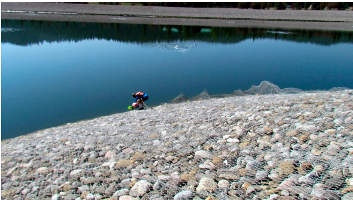
Figure Box 22-1 - Beginning a fluorescein introduction into a sewage pond. The damaged gabions are shown to the right of the person introducing dye.
