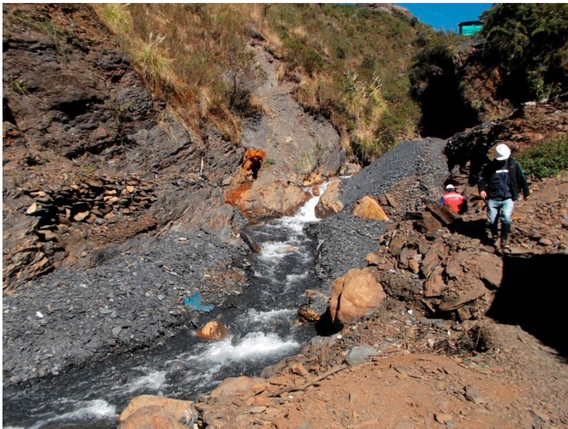
Figure 29 - Acid mine drainage from a small gold mine in southern Peru. Illegal mining operations often use mercury for gold recovery, and dangerous concentrations of it are commonly found in streams such as the one shown in this photo. Also note the black tailings along the stream from this and other mines.
