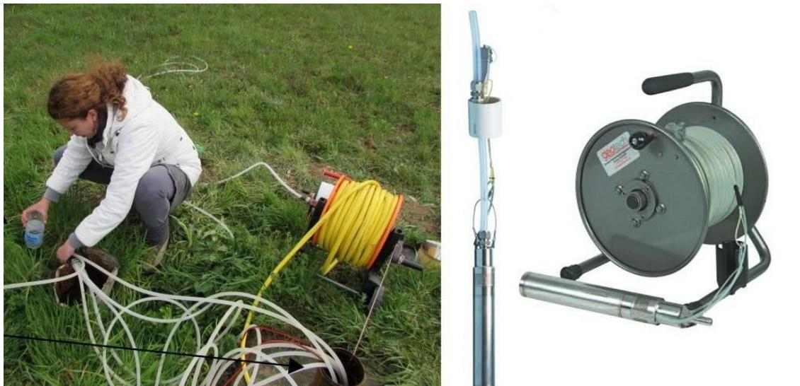
**Figure 87** - Water sampling using a small submersible pump (photographs courtesy of S. Milanović).
