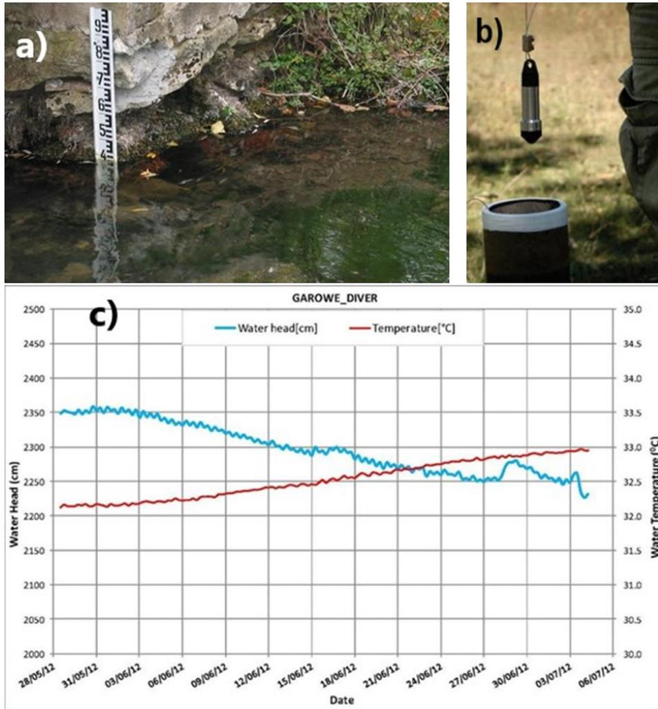
**Figure 85** - Water level monitoring. a) Classic staff gauge and b) water level/temperature recorder with data logger. c) A graph showing two months of data on water level and temperature, digitally recorded in one borehole in the karst of Somalia.
