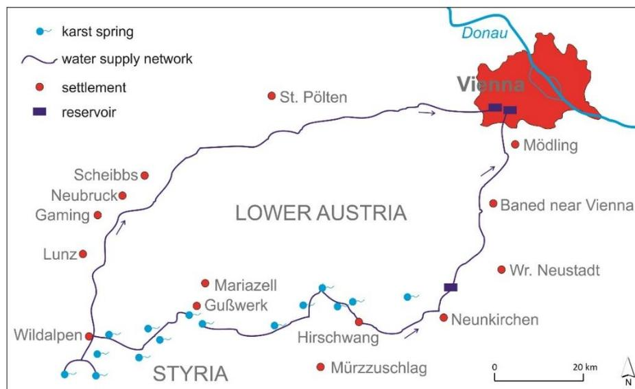
**Figure Box 21-2** - Vienna is supplied with drinking water from karst springs via two long-distance pipelines with a combined length of more than 200 km.
