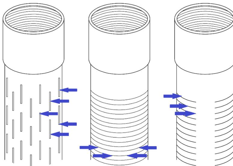
**Figure 59** - Several types of screens with threaded joints (from left to right: slotted screen, continuous slot wire-wound screen, and screen with plain surfaces).
