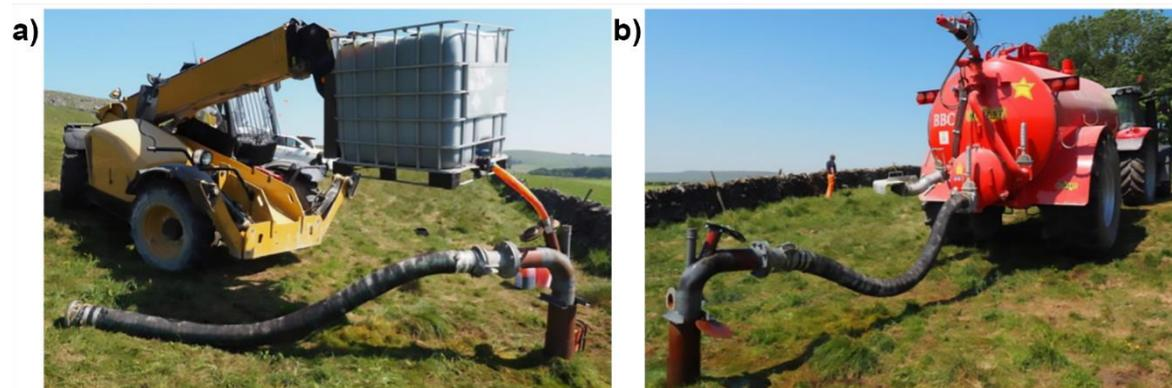
**Figure Box 11-2** - Tracer injection into drilled boreholes: a) dye, dissolved in water, discharging from a 1,000 L container into the borehole; b) bowser used to flush dye after injection (photographs by J. Gunn).
