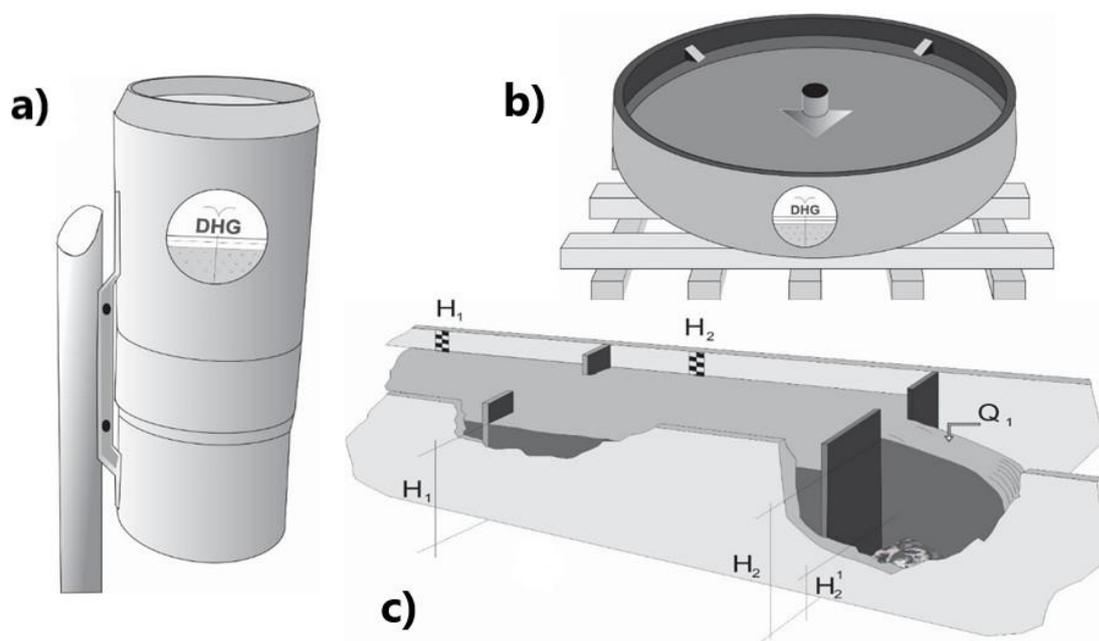
**Figure Box 22-1** - Common devices for measuring water budget elements: a) storage rain gauge, b) evaporation pan, and c) two, successive, rectangular-notch, weirs with control gauges for measuring water heights ( $H$ ).
