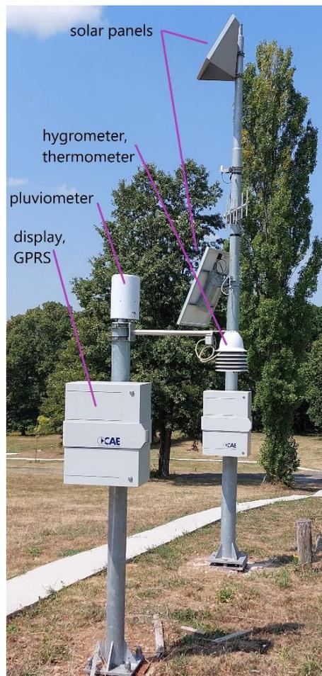
**Figure Box 22-2** - Automatized and remotely controlled mini meteorological station (rainfall, humidity, air temperature). Snow is melted using energy provided by solar panels to convert it into a water column (photograph by Z. Stevanović).
