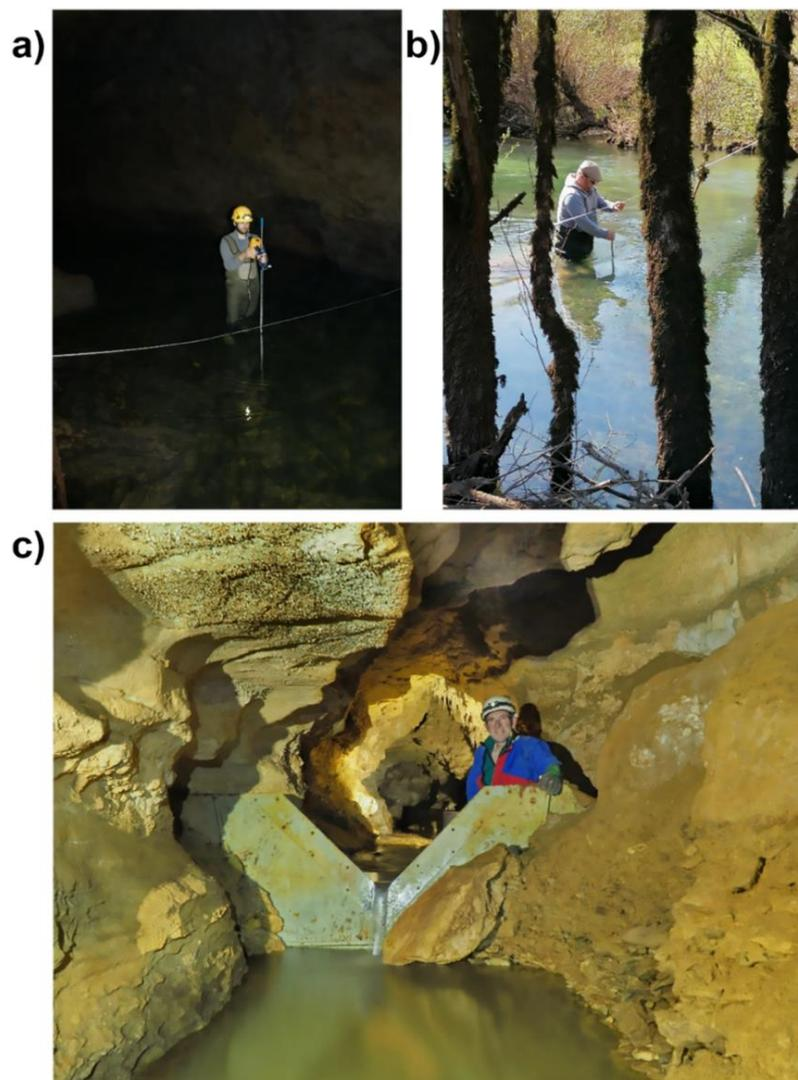
**Figure Box 22-3** - Measurement of stream discharge. Use of current meters to measure stream velocity so that discharge can be calculated using the velocity-area method, a) in a cave (photograph by N. Ravbar) and b) in a surface river (photograph by Z. Stevanović). c): A sharp-crested 90-degree v-notch weir used to measure discharge in Mangapohue Cave, Waitomo, New Zealand (photograph by J. Gunn).
