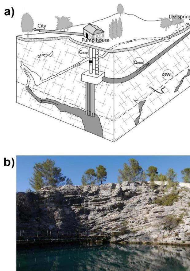
**Figure Box 28-1** – Engineering regulation of Lez spring: a) source and intake scheme (from Montpellier waterworks leaflet, modified by Stevanović, 2015). Legend: GWL = groundwater level;  $Q_{\text{expl}}$  = groundwater flow extracted for water supply of the city;  $Q_{\text{eco}}$  = guaranteed groundwater ecological flow diverted to spring orifice. b) photograph of spring (by N. Goldscheider).
