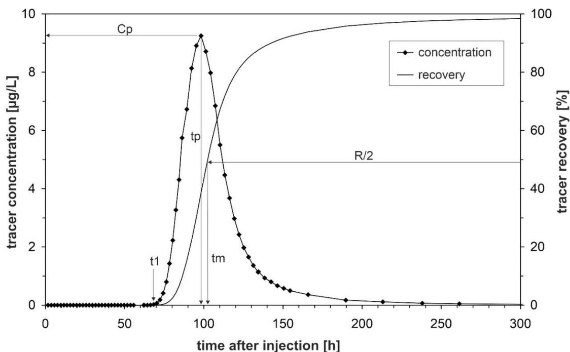
**Figure Box 13-1** - Example of a tracer breakthrough curve (BTC) with illustration of parameters that can be obtained from this curve, as explained in the text (modified after Goldscheider et al., 2008).
