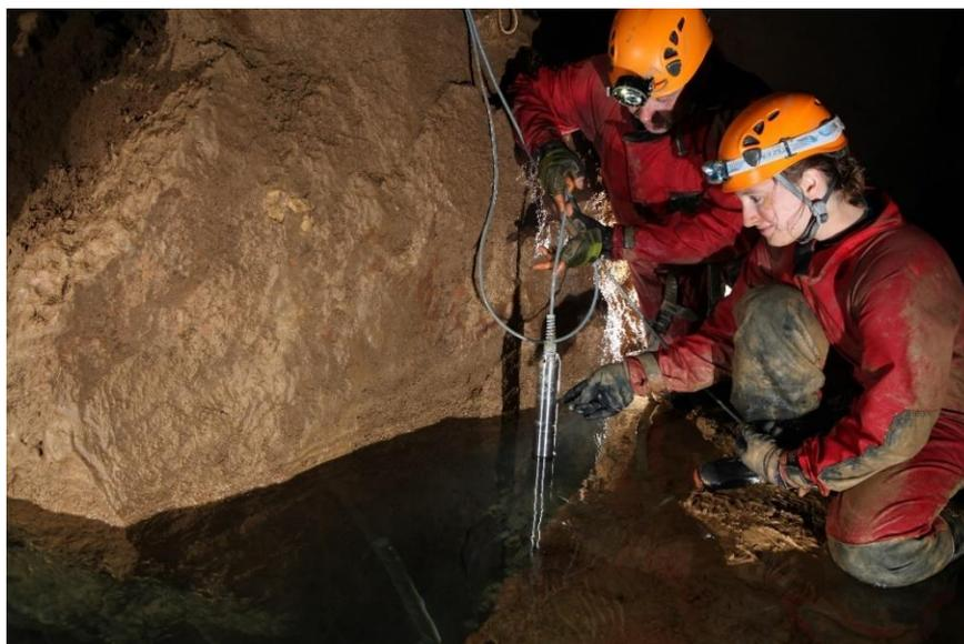
**Figure 88** - Installation of field fluorimeter (Blue Cave, Swabian Alb, Germany) for an in-cave dye-tracer test (photograph courtesy of A. Kücha).
