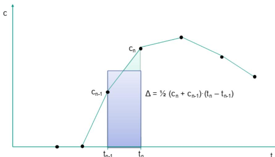
**Figure Box 13-2** - Illustration of the quantification of tracer recovery from a BTC. The curve is sliced in individual segments that can be approximated as rectangles, which are then summed up. Finally, the surface below the BTC is multiplied by the discharge. Legend:  $t$  = time,  $c$  = concentration,  $n$  and  $n-1$  = sample numbers,  $\Delta$  = area of an individual rectangular slice of the BTC.
