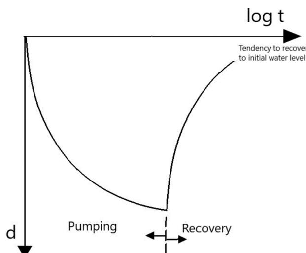
**Figure 60** - Diagram of pumping test drawdown versus time [ $d = f(\log t)$ ] and groundwater recovery.
