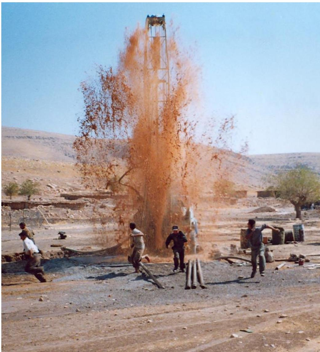
**Figure Box 10-1** - Huge and unexpected free flow with high pressure from a drilled well in the Pila Spi karst aquifer (Kani Shaya, northern Iraq; photograph courtesy of R. Karwan).
