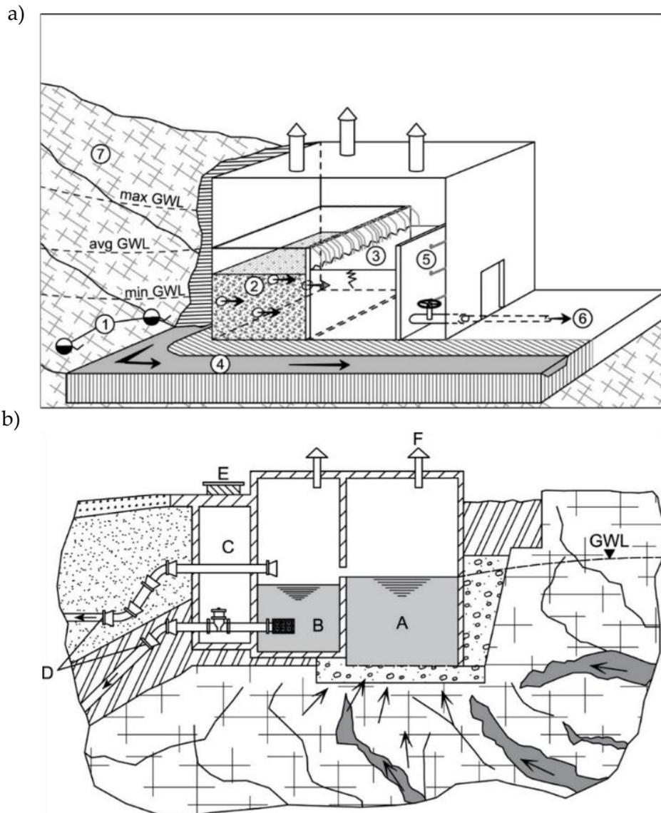
**Figure Box 18-1** - Capture structures for a) a descending karst spring and b) an ascending spring (modified from Stevanović, 2015). Legend: 1. Small seepage springs, 2. Reservoir of clean water, 3. Overflow, 4. Evacuation canal, 5. Valve, 6. Delivery pipe, 7. Karst aquifer, A. Sediment box, B. Reservoir of clean water, C. Maintenance room with valves, D. Overflow and delivery pipes, E. Entrance, F. Vent.
