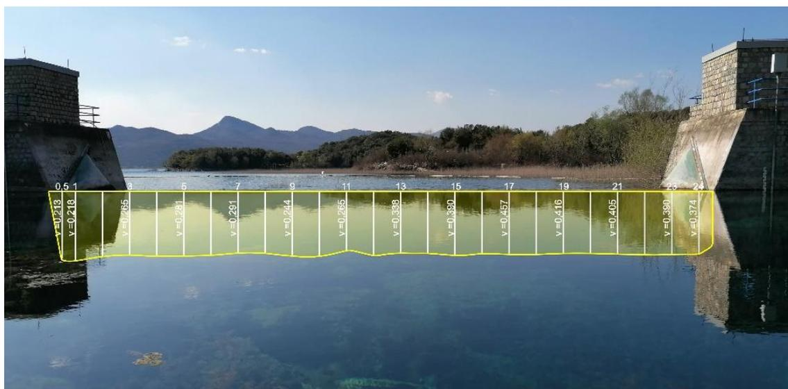
**Figure 84** - Weir on the karst spring Bolje Sestre (Skadar Lake, Montenegro). The velocities at 24 verticals with known depths are measured by an observer and the discharge is calculated using the velocity-area method. A staff gauge, installed for control readings of water level in the intake, can be seen in the right corner (photograph by Z. Stevanović)
