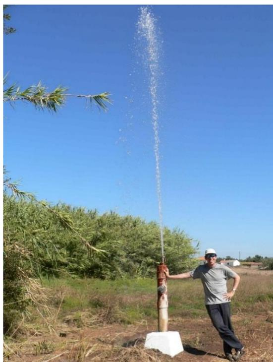
**Photograph Album 72** - Groundwater monitoring well with open cap in an artesian karst aquifer in Portugal, illustrating that the potentiometric surface in the aquifer is above the land surface (photograph by N. Goldscheider).
