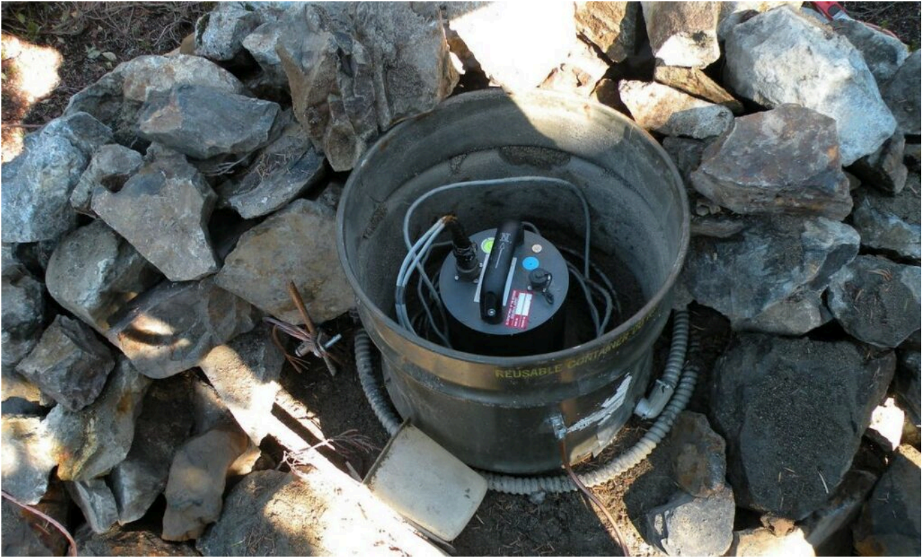
Figure 7.5.1 A Seismometer Installed in a Vault Above Ground at Mount Baker, Washington.
