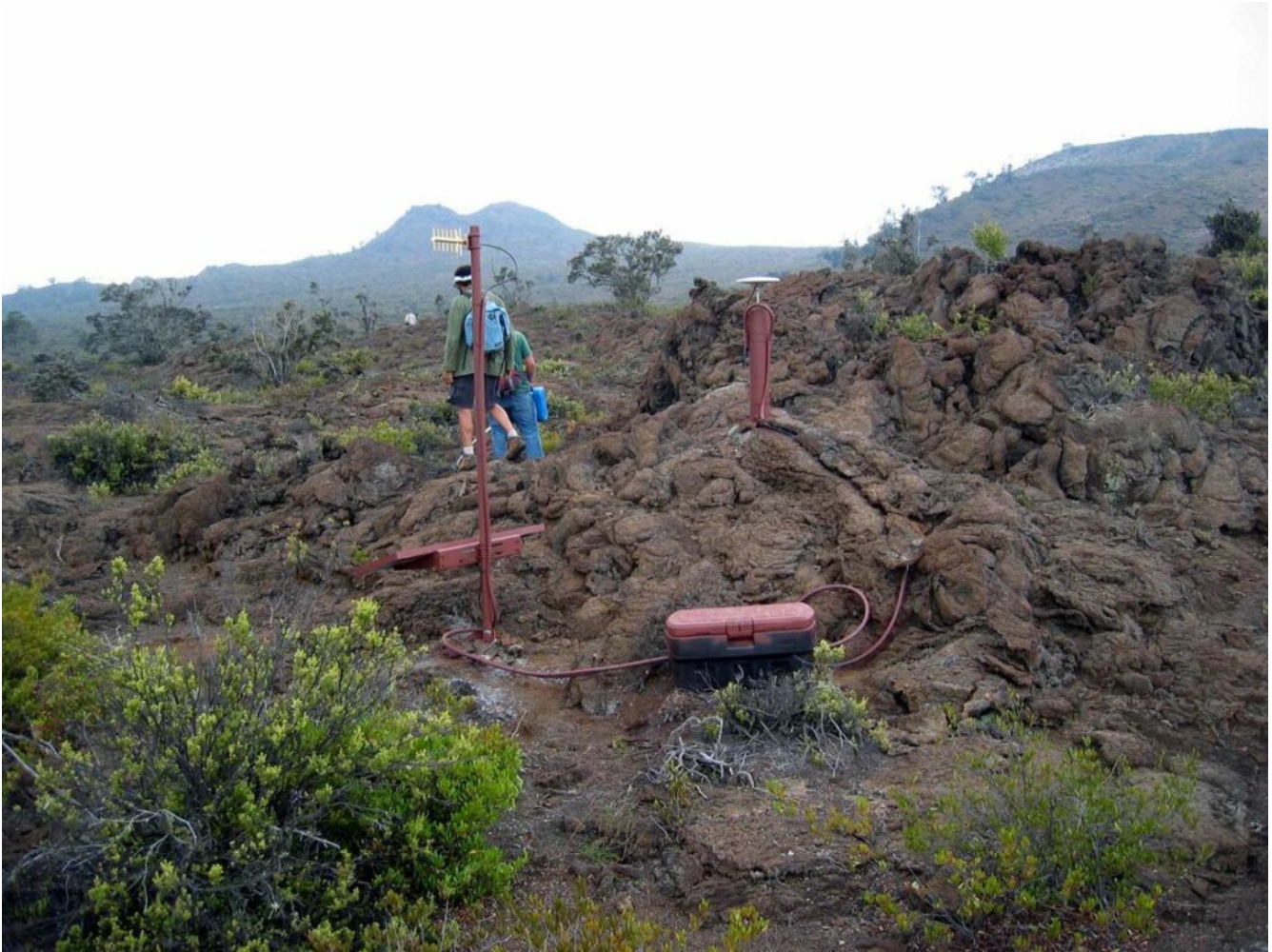
Figure 7.5.2 A GPS Unit Installed at Hualalai Volcano, Hawaii. The dish-shaped antenna on the right is the GPS receiver. The antenna on the left is for communication with a base station.
