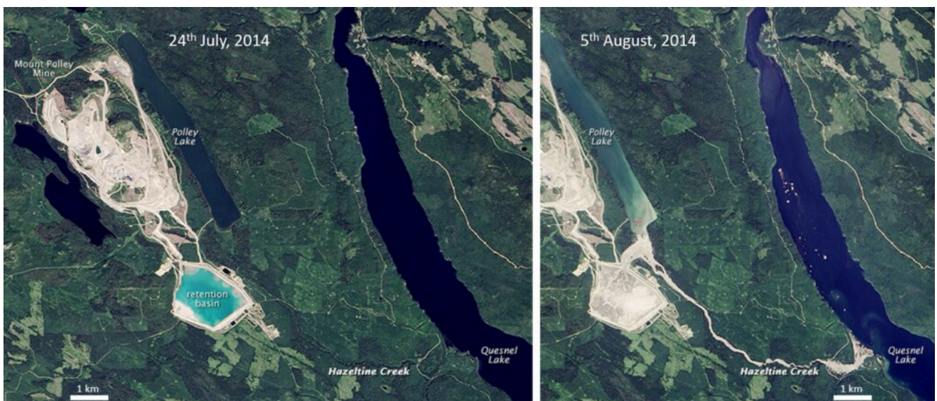
Figure 8.2.4 The Mt. Polley Mine Area Before (left) and After (right) to the Dam Breach of August 2014. The tailings were stored in the area labelled “retention basin”.
