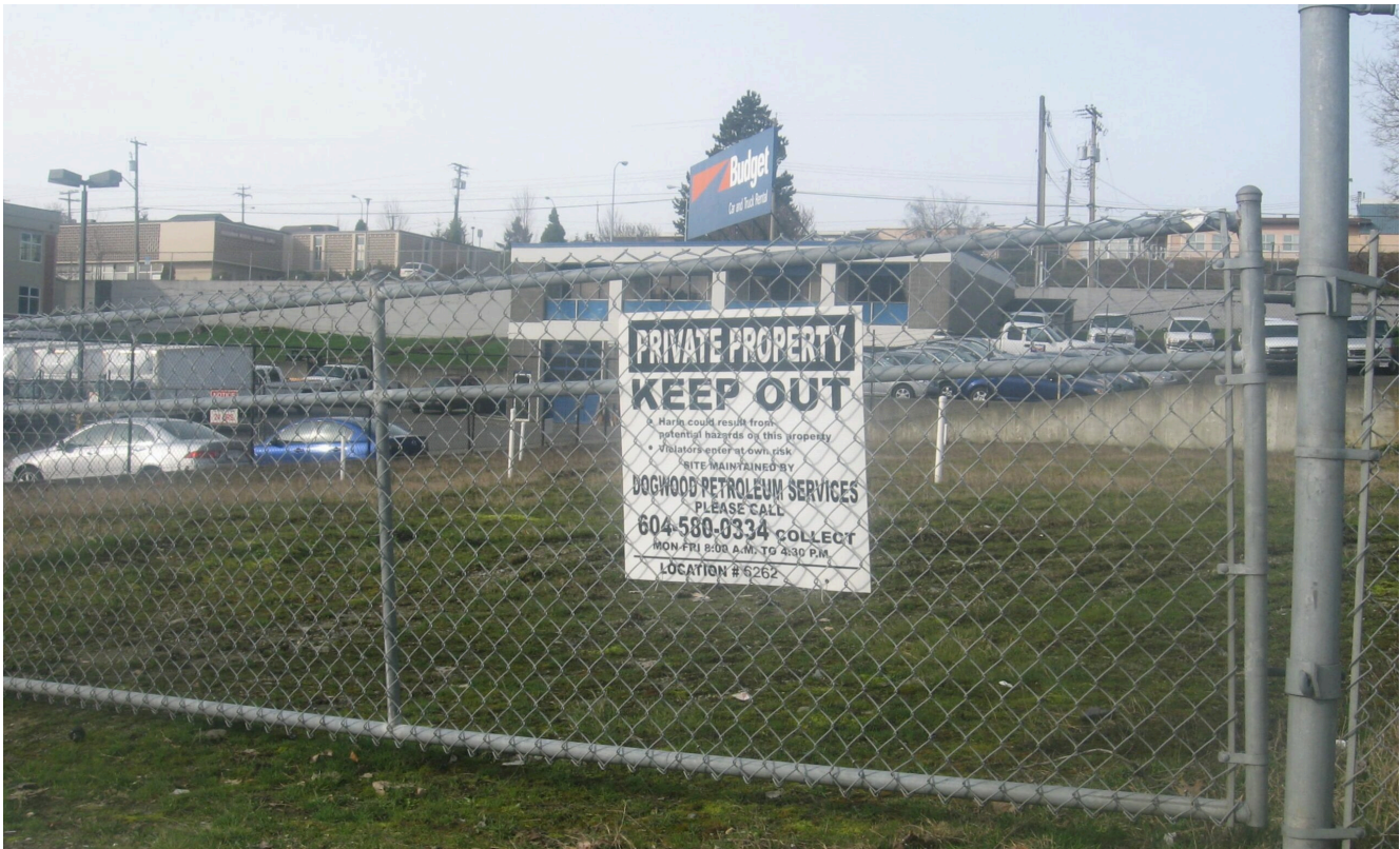
Figure 11.2.6 The Site of a Filling Station With Leaking Underground Storage Tanks. The white pipes are groundwater monitoring wells.
