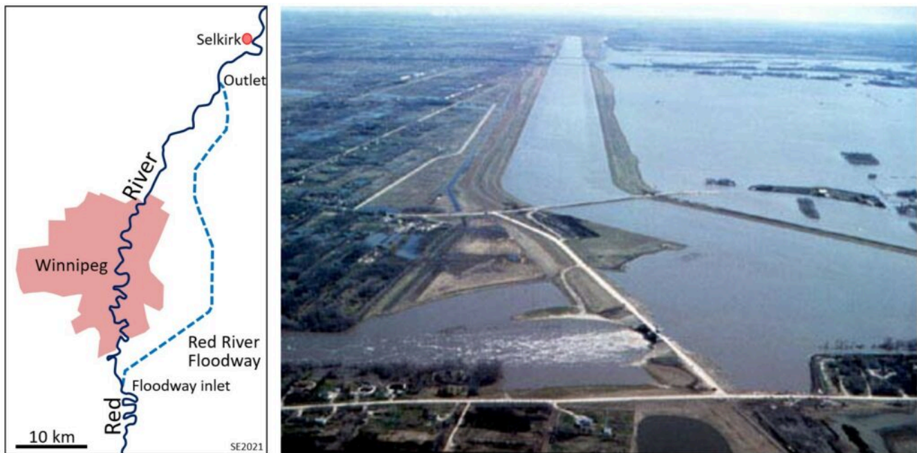
Figure 13.3.4 Map of the Red River Floodway Around Winnipeg, Manitoba (left), and Aerial View of the Southern (inlet) End of the Floodway (right) Taken During the 1997 Flood.
