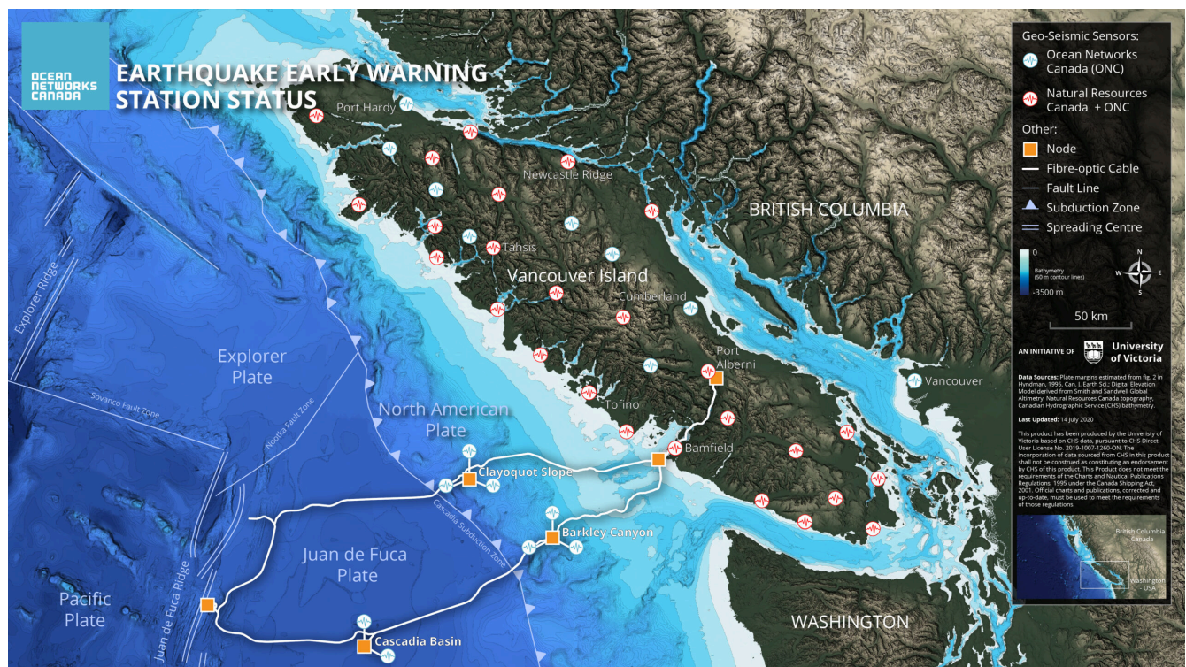
Figure 6.5.3 Ocean Networks Canada Earthquake Early Warning System for Southwestern British Columbia
