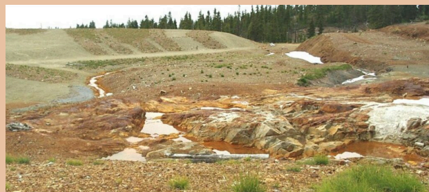
Figure 8.2.5 Waste Rock and Acid-Rock Drainage at the Mt. Washington Mine, BC
