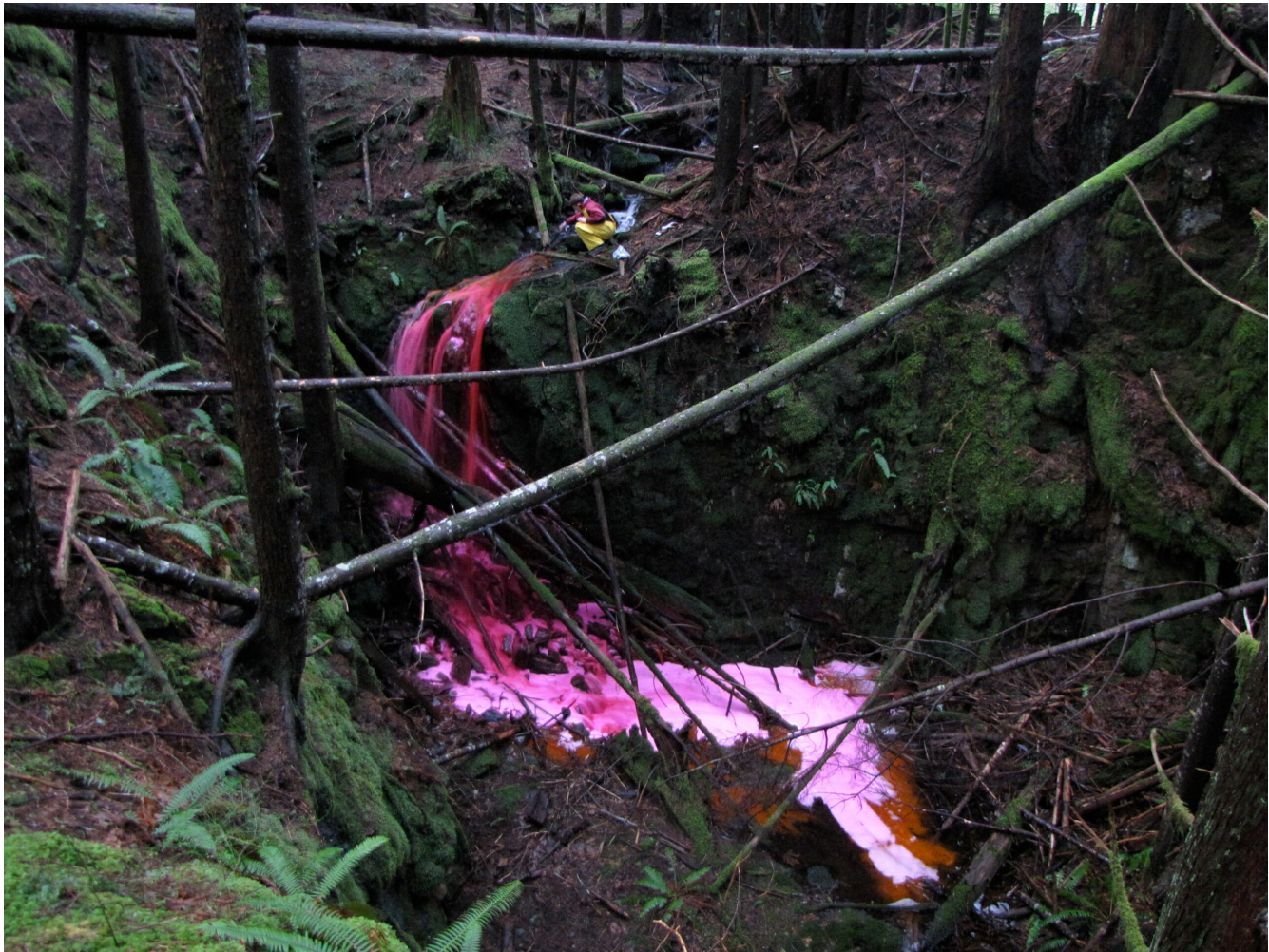
Figure 12.3.8 Introduction of Rhodamine Dye into a Sinking Stream, Vancouver Island, BC
