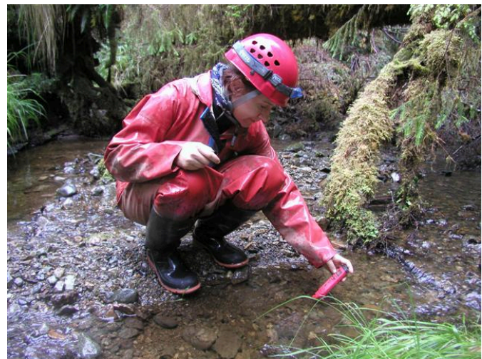
Figure 12.3.7 Measuring Water Conductivity in a Spring
