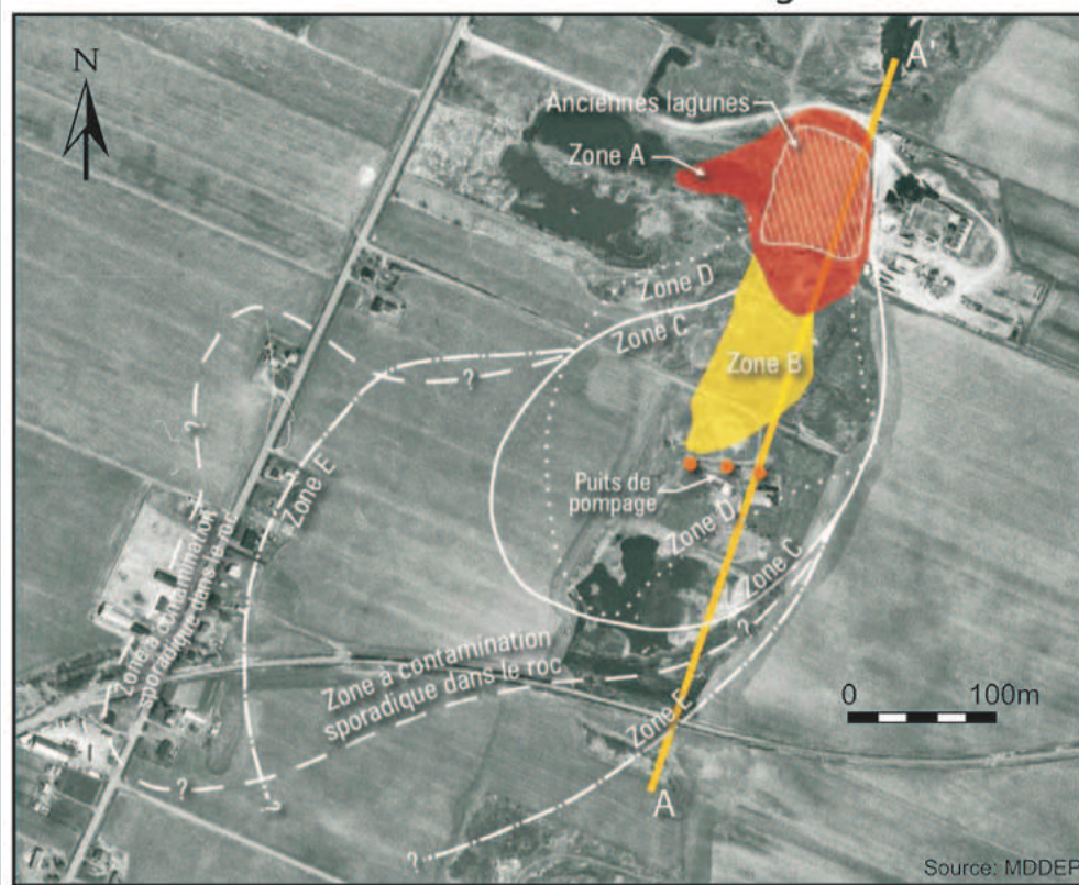
Figure 13.38 Plan view of the contaminated plume in the Mercier Lagoons (Source: Côté et al., 2006).
