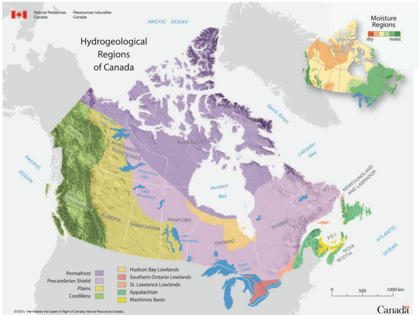
Figure 8.1 Hydrogeological regions. Map of nine colour-coded hydrogeological regions, identified by major geological domains, draped on a digital elevation model of Canada (see relief features). Moisture deficit or surplus is indicated by generalized dry (red) and moist climate regions (green) in inset map.
