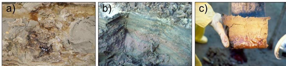
**Figure 5** - Photographs of DNAPL encountered in the subsurface showing a) and c) DNAPL at sufficient saturation to flow out of the sand and (b) DNAPL at insufficient saturation to flow out of the sand. Pink- and red-colored DNAPL is the result of dye added as part of field experiments (photographs by B. Kueper).
