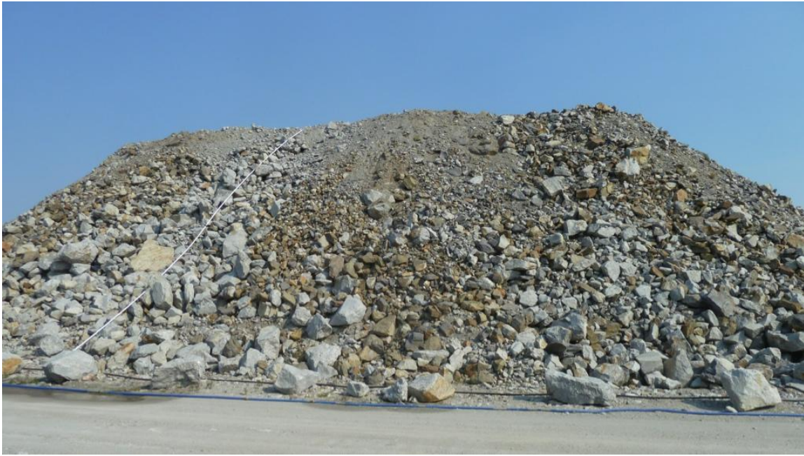
Figure 11 - A 15 m high waste rock test pile built by end dumping, illustrating a broad range in particle size and particle segregation on the tip face.
