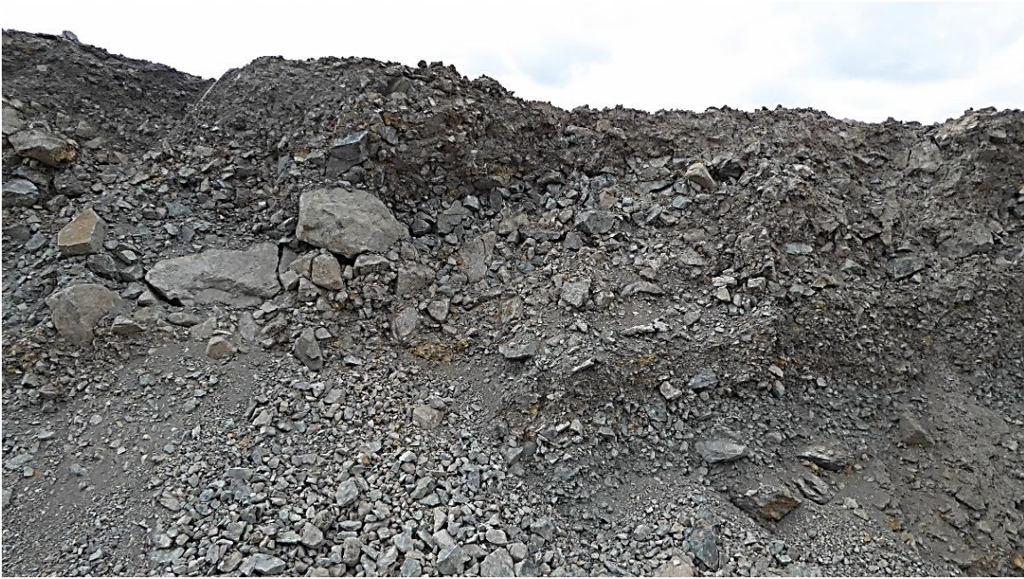
Figure 13 - Excavation in a waste rock stockpile. Vertical face approximately 3 m in height. In this region of the stockpile, it is anticipated matrix flow would be dominant process, but the photo also shows in the upper center a region of open voids not infilled with finer grained materials where the saturated hydraulic conductivity is likely to be much greater.
