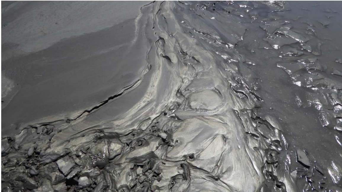
Figure 2 - A deposit of mill tailings in an active deposition area, showing a zone of fine sands in the left of the photo, and a zone of silt-sized tailings to the right. The ribbons in the deposit with a metallic luster are where sulfide minerals were concentrated during sediment transport. Scale of view is approximately 2 meters laterally.
