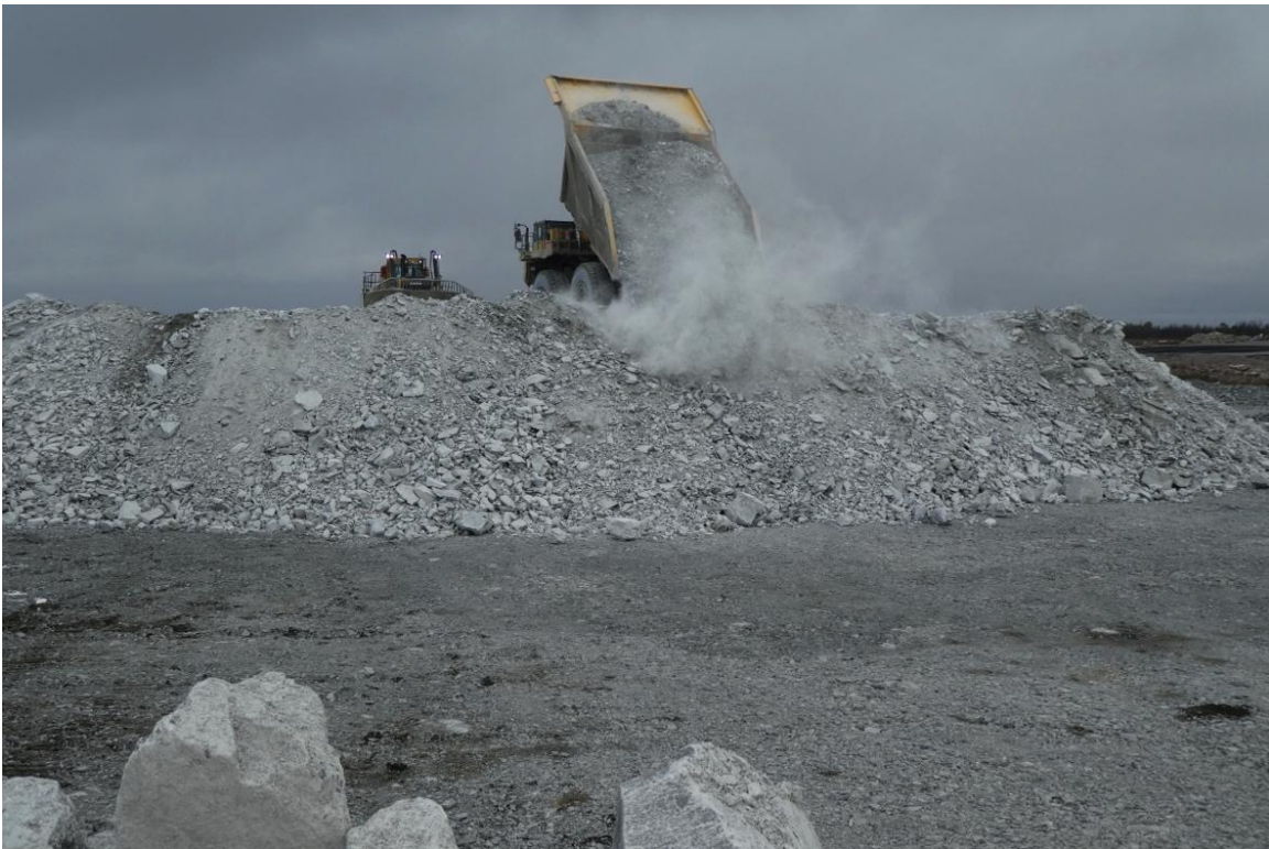
Figure 3 - Waste rock from an open pit operation has a wide range in particle size, and significant variability from one location to the next within the stockpile.
